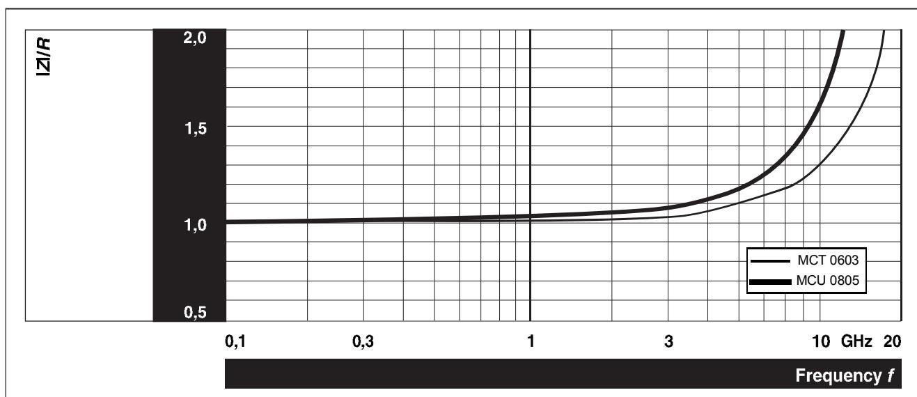
Fig.9  $|Z|/R$  for 49,9  $\Omega$  chip resistor.
