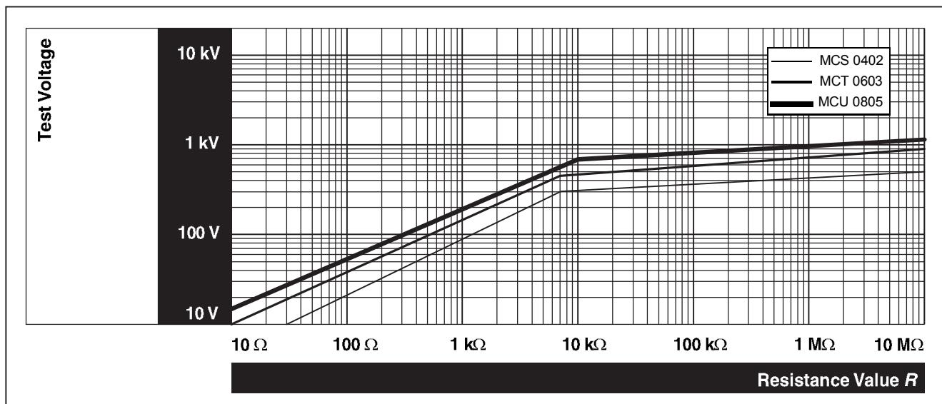
Fig.7 Pulse load rating in accordance with IEC 60115-1 clause 4.27; 10 µs / 700 µs; 10 pulses at 1 minute intervals; for permissible resistance change 0,5%.
