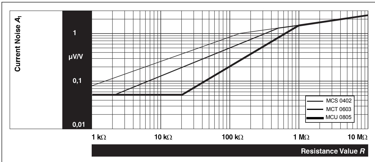
Fig.8 Current noise  $A_1$  in accordance with IEC 60195.**RF-behaviour**
