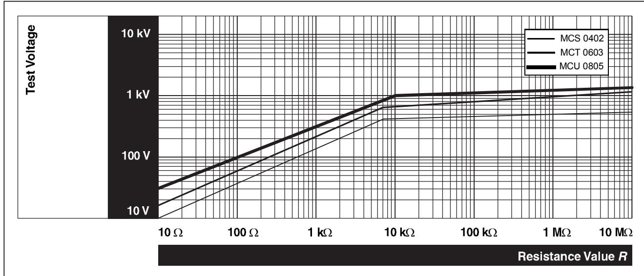
Fig.6 Pulse load rating in accordance with IEC 60115-1 clause 4.27; 1,2 µs / 50 µs; 5 pulses at 12 s interval; for permissible resistance change 0,5%.
