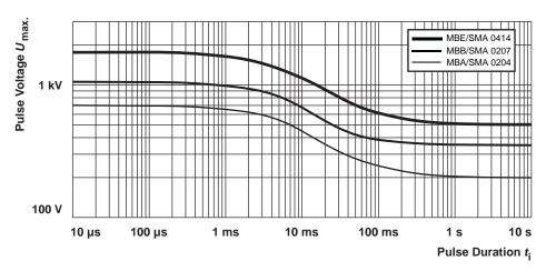
Maximum pulse voltage, single and continuous pulses; for permissible resistance change equivalent to 8000 h operation.
