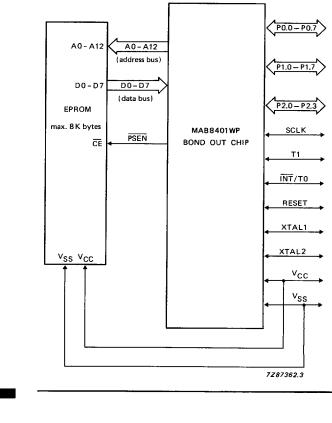
Fig. 3a Connection of EPROM to 'Piggy-back' package MAB8401B.
