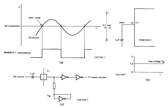
Figure 9 Zero-cross detection circuitry; (a) input waveform, (b) input diagram, (c) on-chip self-stabilized bias.
