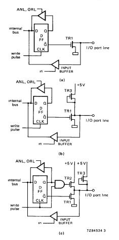
Fig. 7 Quasi-bidirectional I/O interface with (a) open drain output without pull-up transistor, (b) open drain output with pull-up transistor, (c) push-pull output with pull-up transistor.
