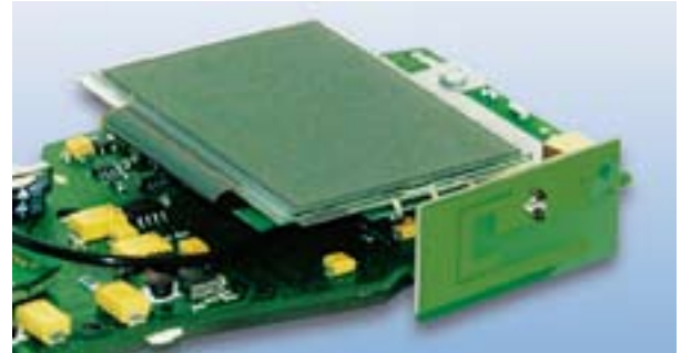
Example for a mobile terminal with embedded GSM antenna
