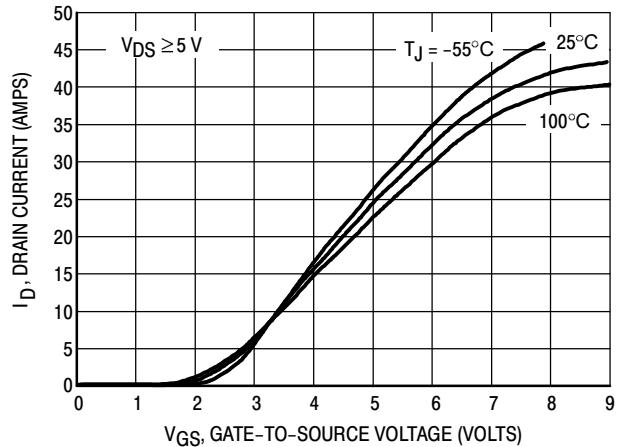
Figure 2. Transfer Characteristics
