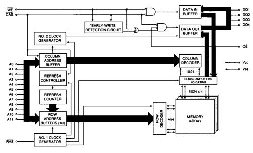
\*NOTE: WE LOW prior to CAS LOW, EW detection circuit output is a HIGH (EARLY-WRITE) CAS LOW prior to WE LOW, EW detection circuit output is a LOW (LATE-WRITE)
