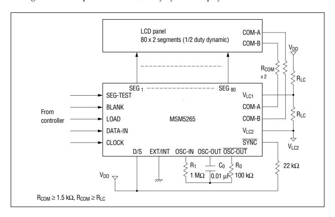
3) Cascade connections for MSM5265s in the static display mode
