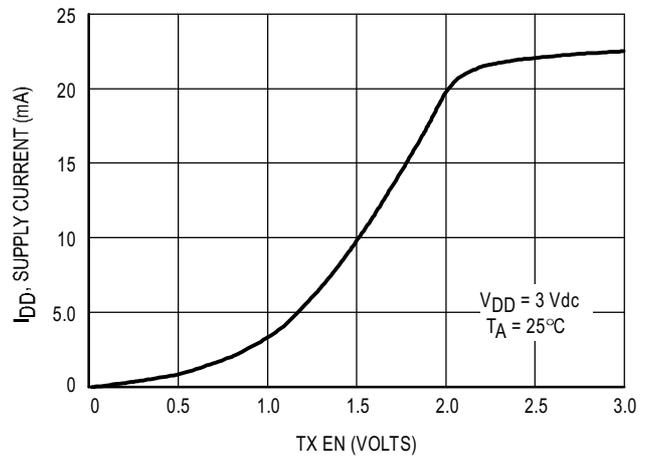
**Figure 17. Supply Current versus Transmit Enable Voltage**
