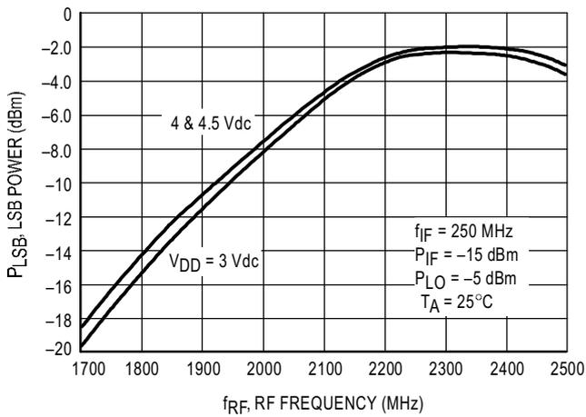
**Figure 16. Lower Side Band Power versus RF Frequency**
