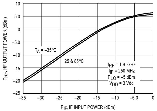
Figure 9. RF Output Power versus IF Input Power
