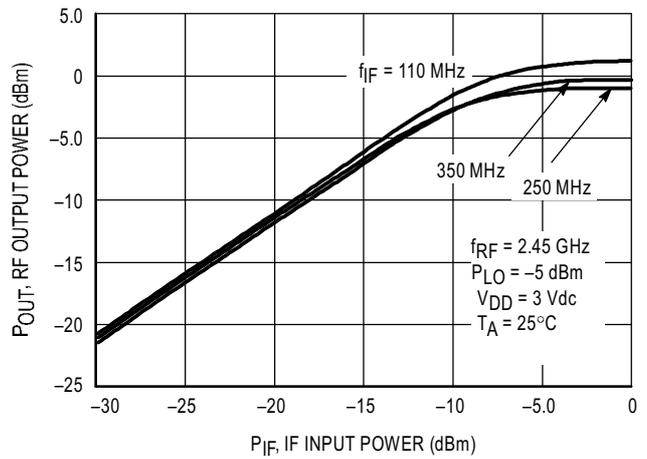
Figure 11. Output Power versus IF Input Power
