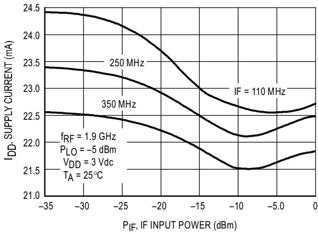
**Figure 14. Supply Current versus IF Input Power**
