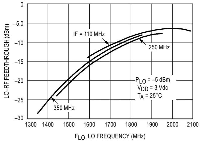
**Figure 15. LO to RF Feedthrough versus LO Frequency**
