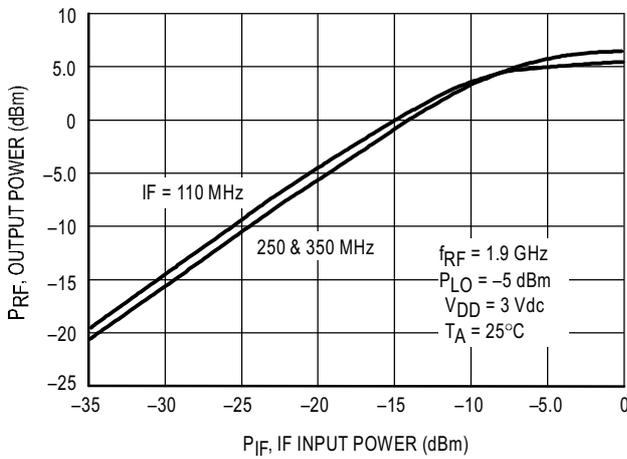
Figure 10. RF Output versus IF Input Power
