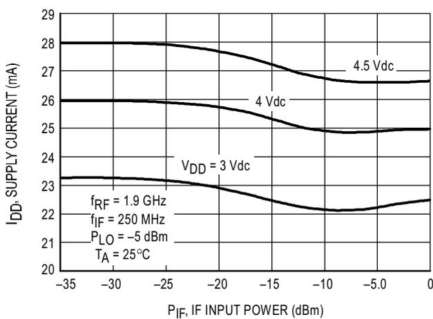
Figure 12. Supply Current versus IF Input Power
