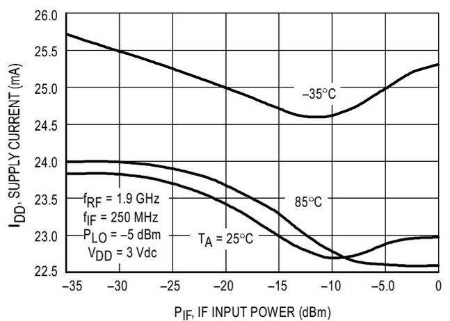
Figure 13. Supply Current versus IF Input Power
