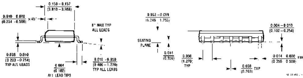
**14-Lead Small Outline Integrated Circuit (SOIC), JEDEC MS-120, 0.150" Narrow Body
