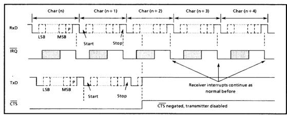
Figure10. Effect of CTS on Echo Mode operation
