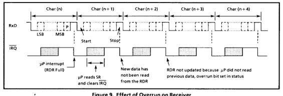
Figure 9. Effect of Overrun on Receiver
