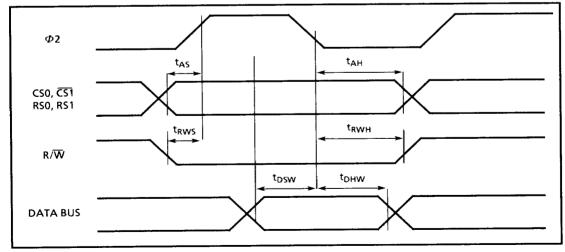
Timing diagram 3 - MPU Write Cycle
