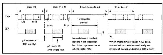
Figure 7. TDR not loaded by Processor
