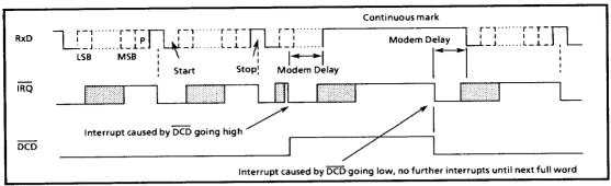
Figure12. Effect of DCD on Receiver
