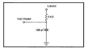
Figure 3. Test load for IRQ
