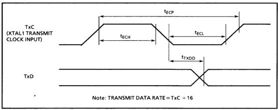
Timing diagram 4 - Transmit Data with External Clock
