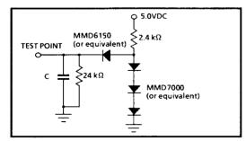
Figure 2. Test load for  $D_0 - D_7$ , TxD,  $\overline{DTR}$  RTS C = 130 pF for  $D_0$ - $D_7$ , C = 30 pF for other outputs
