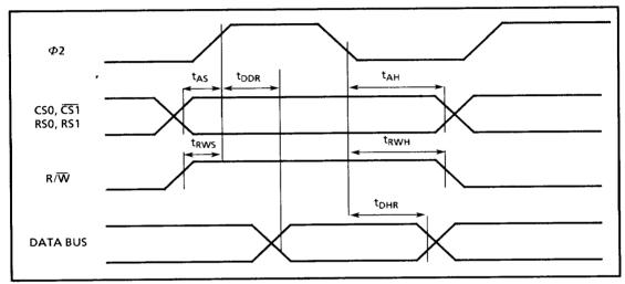
Timing diagram 2 - MPU Read Cycle
