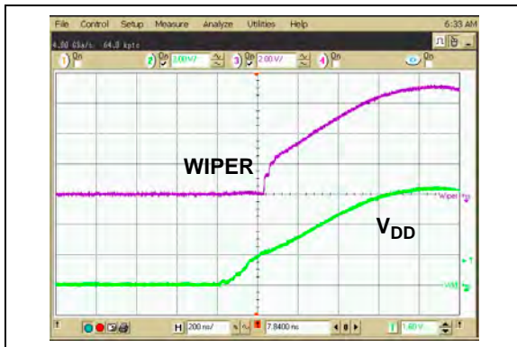
FIGURE 2-45: 50 k \Omega – Power-Up Wiper Response Time.
