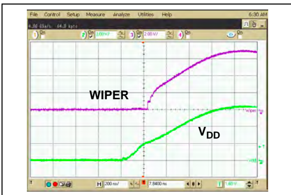
FIGURE 2-14: 2.1 k \Omega – Power-Up Wiper Response Time.
