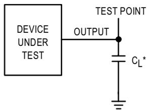
\* Includes all probe and fixture capacitance.
