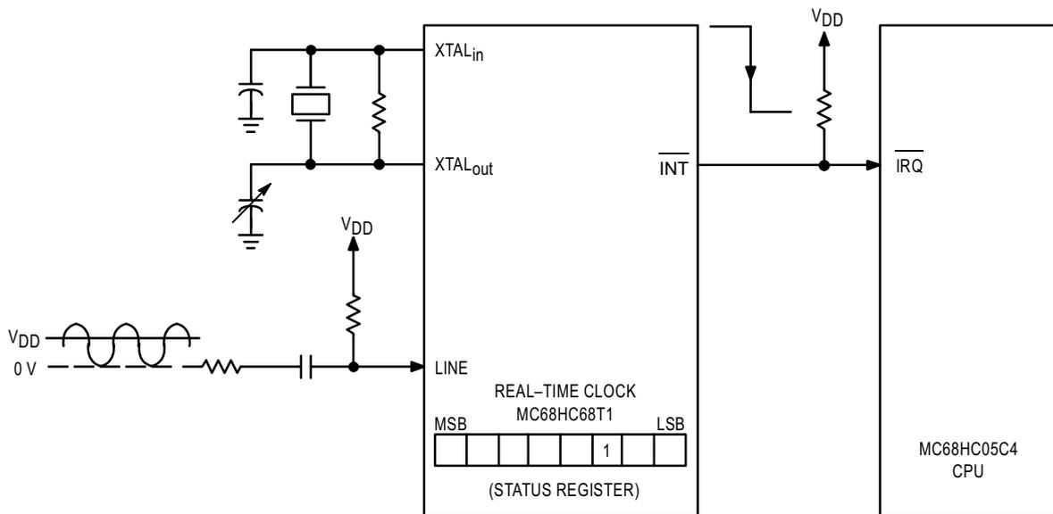
NOTE: A 60 Hz, 10 V p-p sine-wave voltage is an acceptable signal to present at the LINE input pin.
