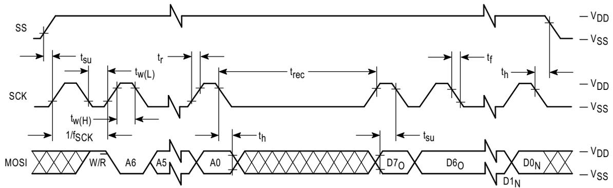
NOTE: Measurement points are  $V_{IL}$  and  $V_{IH}$  unless otherwise noted on the AC Electrical Characteristics table.
