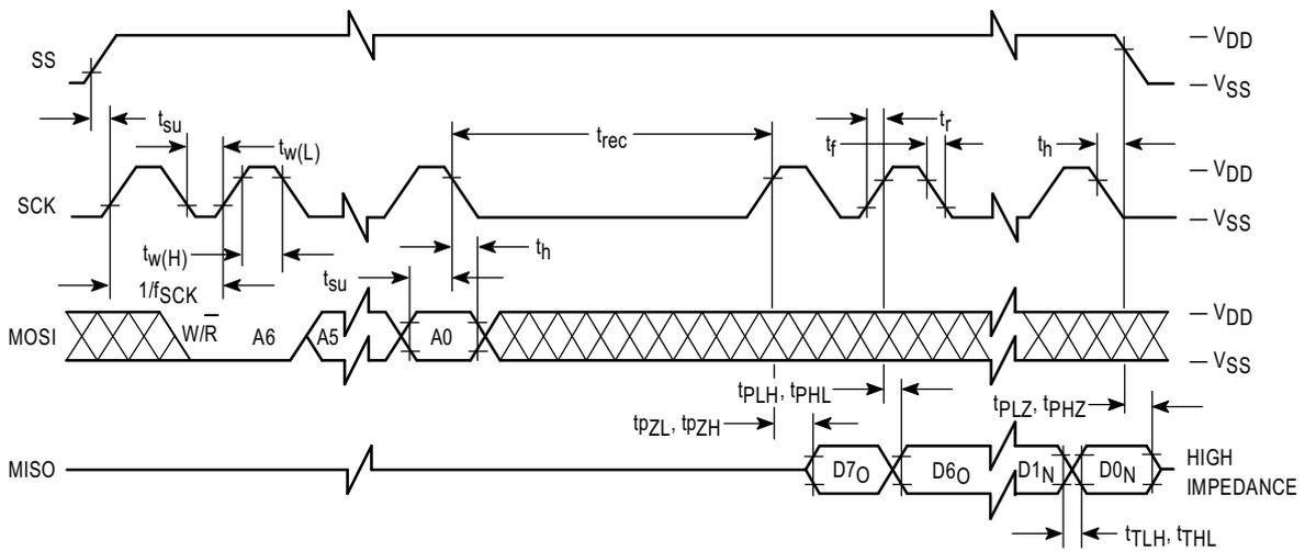
NOTE: Measurement points are  $V_{OL}$ ,  $V_{OH}$ ,  $V_{IL}$ , and  $V_{IH}$  unless otherwise noted on the AC Electrical Characteristics table.
