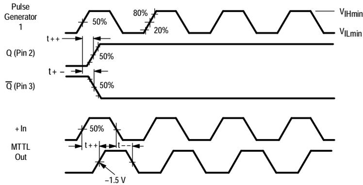
Figure 4. Setup and Release Time Waveforms
