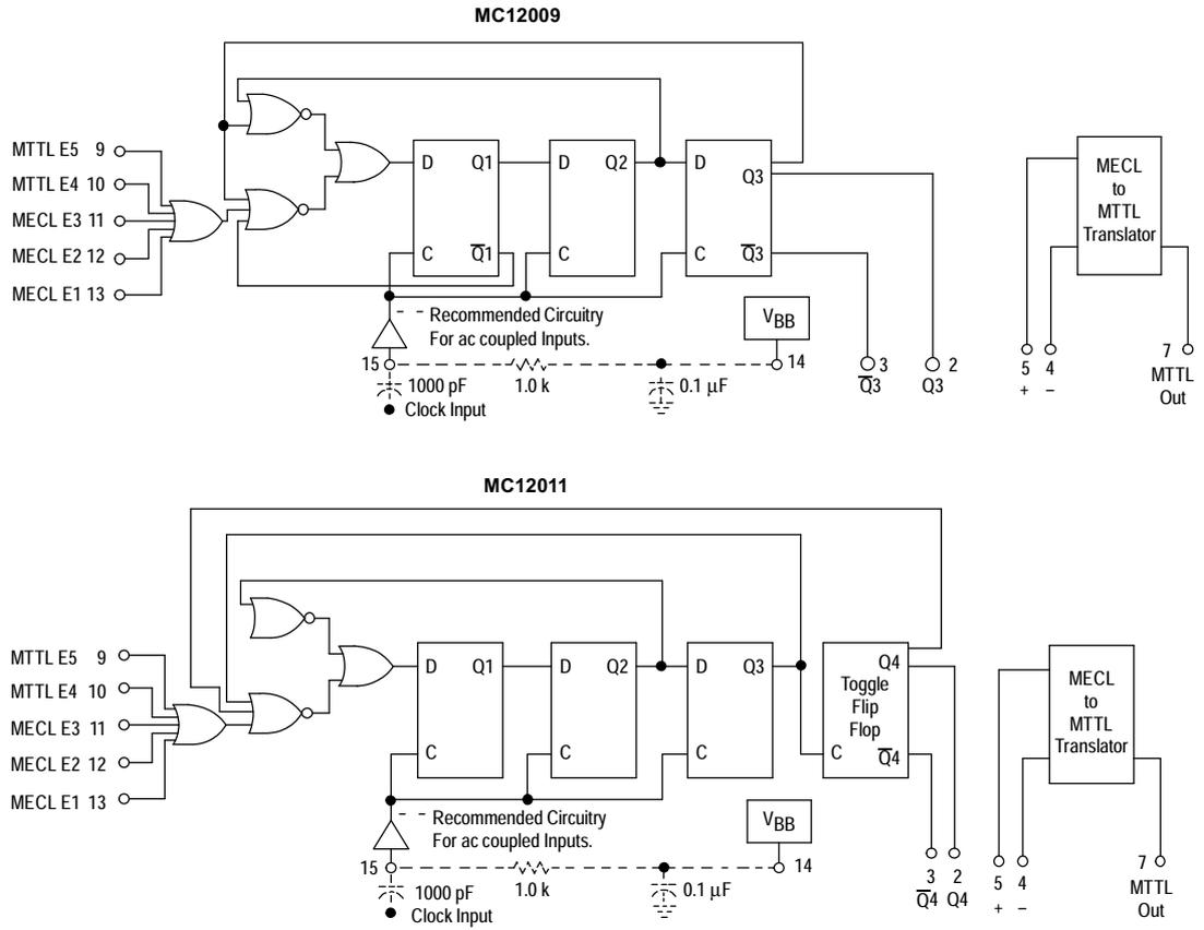
Figure 2. Typical Frequency Synthesizer Application
