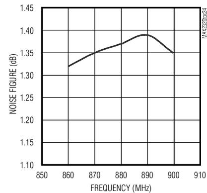
**PCS-BAND HGHL NOISE FIGURE vs. FREQUENCY**
