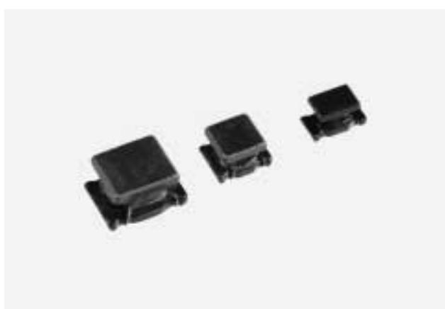
The chip coil LQH/LQN Series comprises subminiature chip inductors wound on a special ferrite core made possible by an automatic winding technique developed by Murata Electronics. These inductors have a high Q at high frequencies and low DC resistance, making them suited for enhancing the performance of electronic circuits in video, communications and audio equipment.
