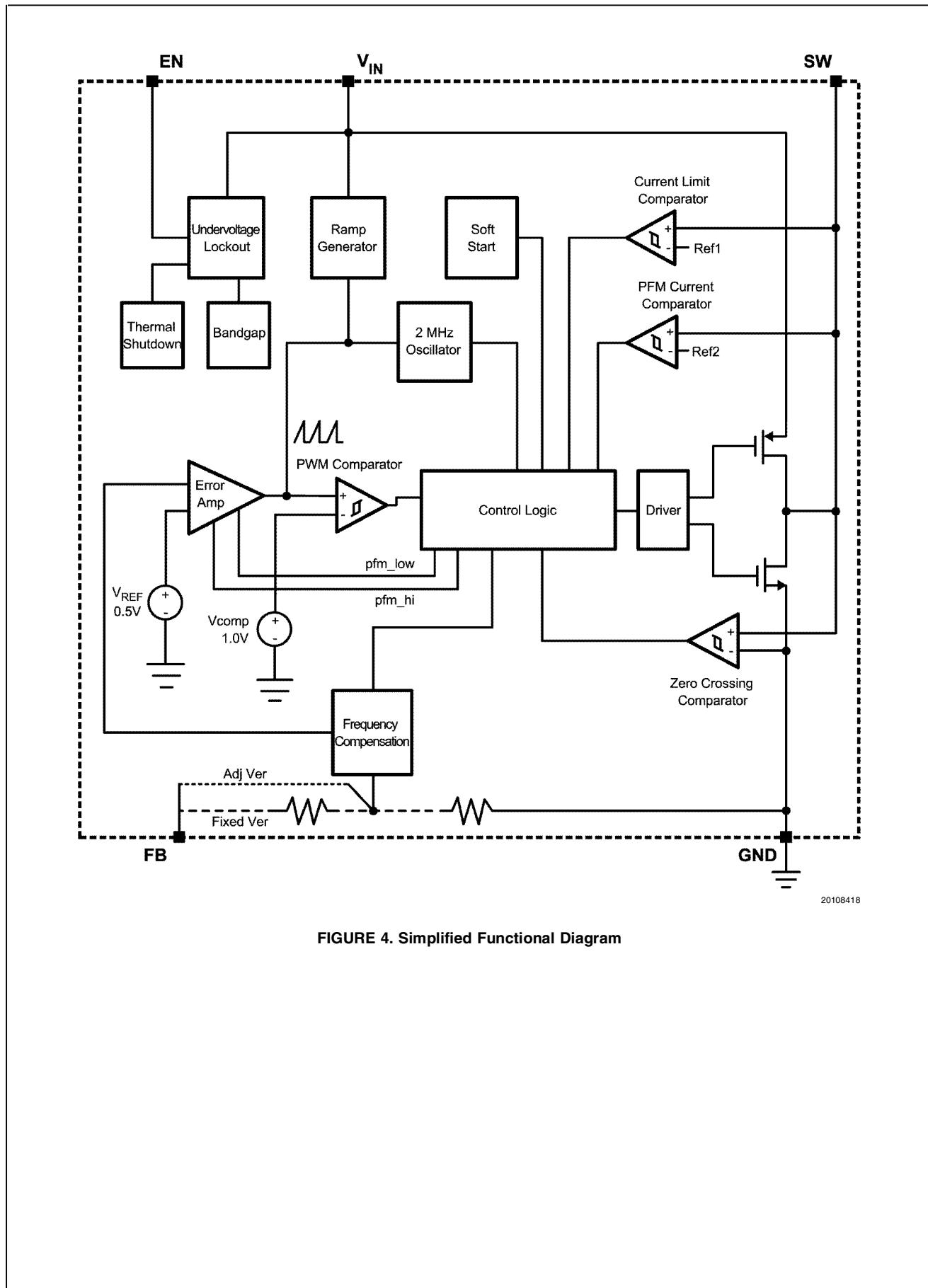
FIGURE 4. Simplified Functional Diagram
