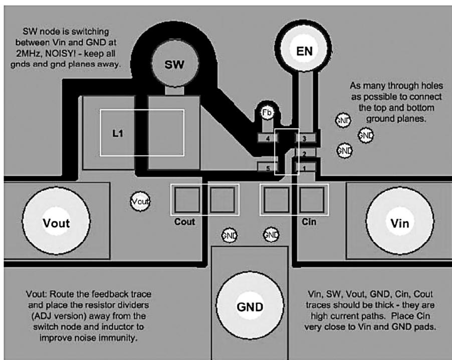
**FIGURE 8. Board Layout Design Rules for the LM3671**
