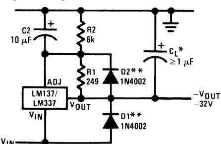
\*When  $C_L$  is larger than 20 μF, D1 protects the LM137 in case the input supply is shorted
