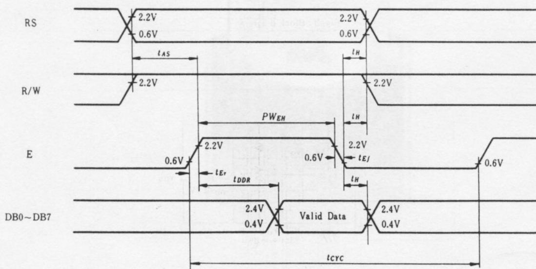
Fig. 6 Interface timing (data read)
