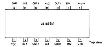
Note) Both GNDs must be connected. P-GND of OUT2 and OUT4 and S-GND of the control section are connected to the pin 7 GND within the IC, and P-GND of OUT1 and OUT3 is connected to the pin 14 GND.
