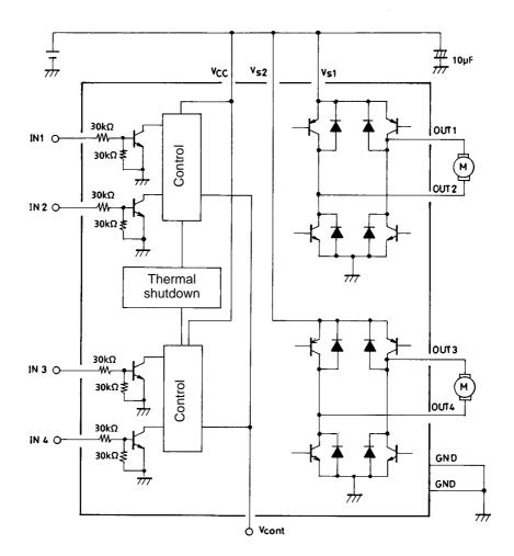
Note: As long as the voltages applied to V<sub>CC</sub>, V<sub>S</sub>1, V<sub>S</sub>2, and IN1 through IN4 are within the limits set by the absolute maximum ratings, there are no restrictions on the relationship of each voltage level in comparison with the others (regarding which is higher or lower). (ex. V<sub>CC</sub> = 3 V, V<sub>S</sub>1, 2 = 2 V, IN1 to IN4 = 5 V)
