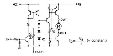
As shown in the above diagram, the Vcont pin outputs the voltage of the band gap Zener  $V_Z+V_F$  (= 1.93 V). In normal use, this pin is left open.
