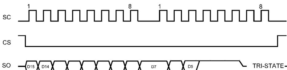
b) Reading Continuous Conversion - Two Eight-Bit Frames 10122315
