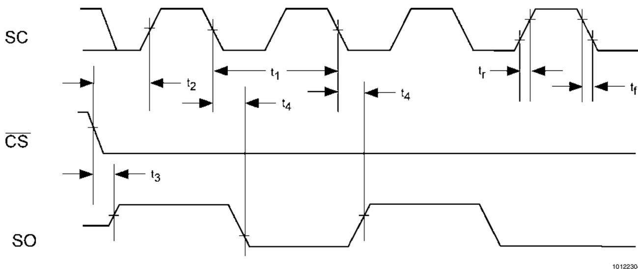
FIGURE 2. Data Output Timing Diagram
