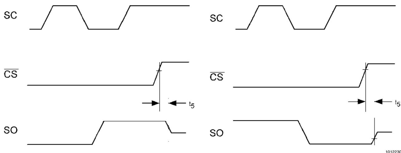
FIGURE 3. TRI-STATE Data Output Timing Diagram
