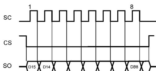
a) Reading Continuous Conversion - Single Eight-Bit Frame 10122314
