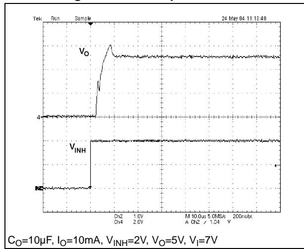
**Figure 22. Start-up time 1.5 A**
