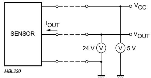
Fig.6 Leakage current test circuit: OUT to GND.
