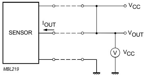
Fig.5 Leakage current test circuit:  $V_{CC}$  to OUT.
