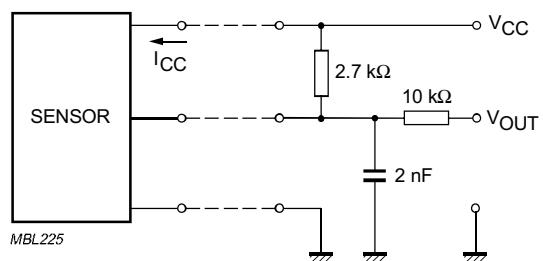
Fig.7 Test and application circuit with additional ceramic capacitor.
