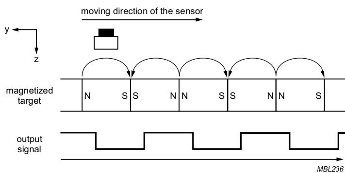
Fig.8 Functional principle.
