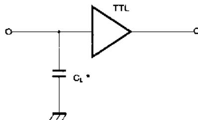
\* Including Scope and Jig Capacitance
