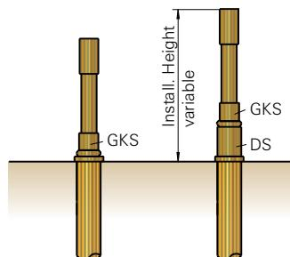
\* Example of usage of a Receptacle with and without Spacer (restrictions see above)
