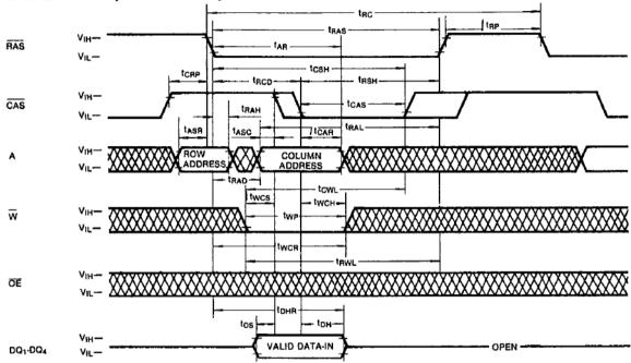
WRITE CYCLE (OE CONTROLLED WRITE)
