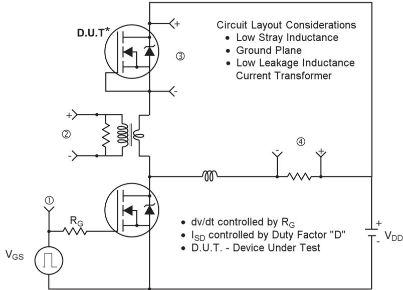
\* Reverse Polarity of D.U.T for P-Channel
