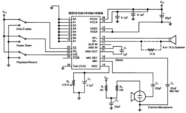
Note: If desired, this pin may be left unconnected (microphone preamplifier noise will be higher). In this case, pin 18 must not be tied to any other signal or voltage.
