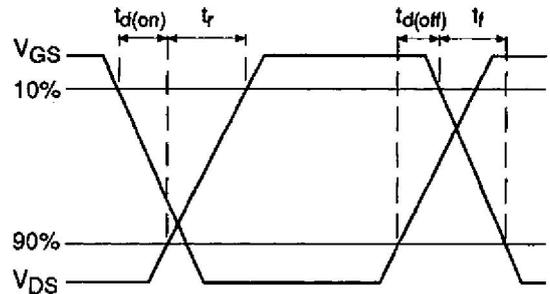
**Fig 10b.** Switching Time Waveforms
