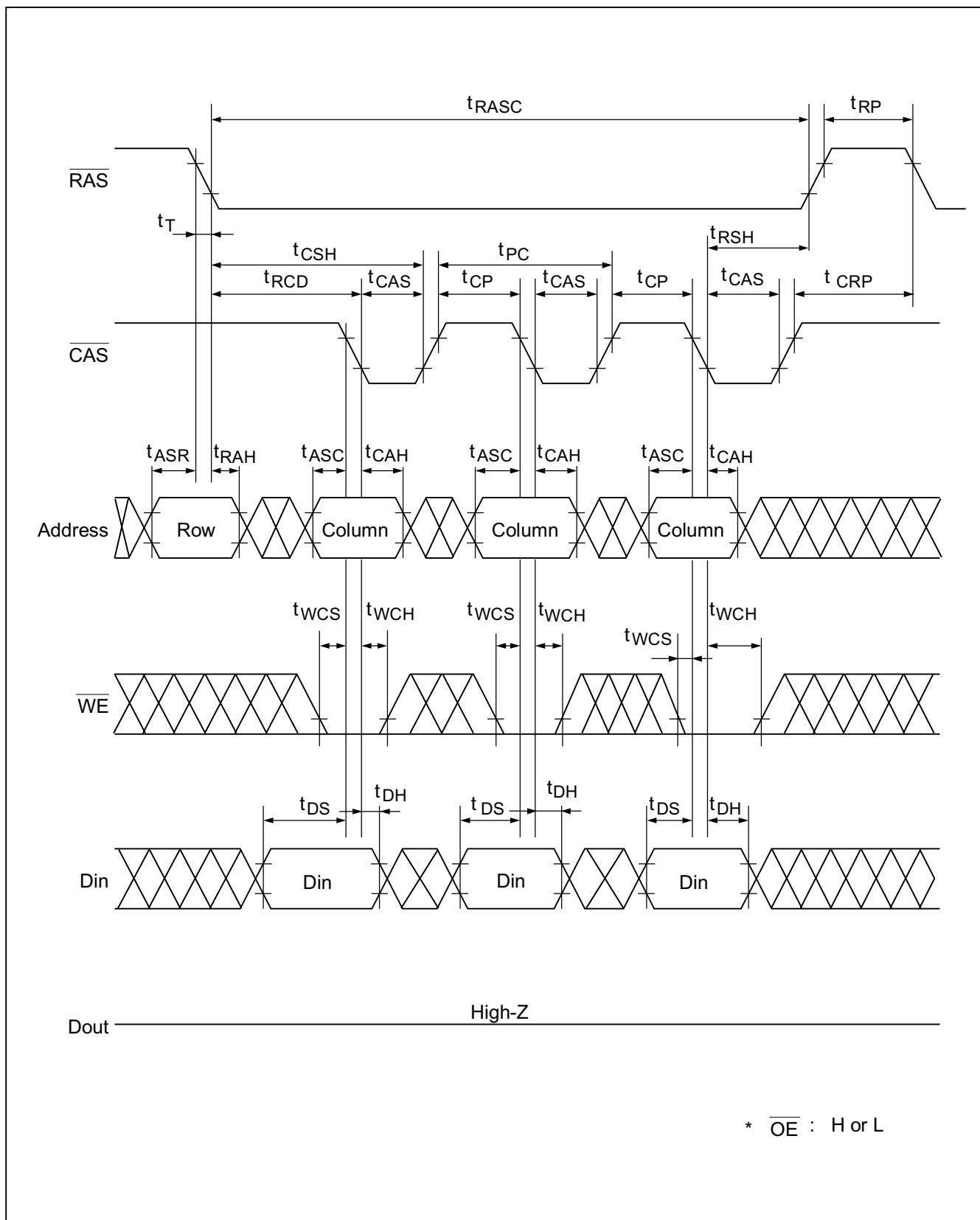
**Fast Page Mode Delayed Write Cycle**
