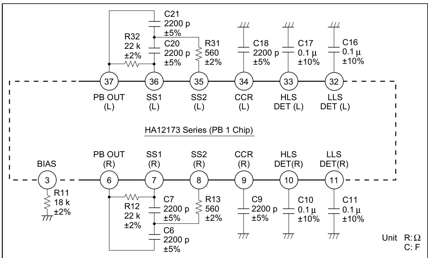
Figure 6 Tolerances of External Components
