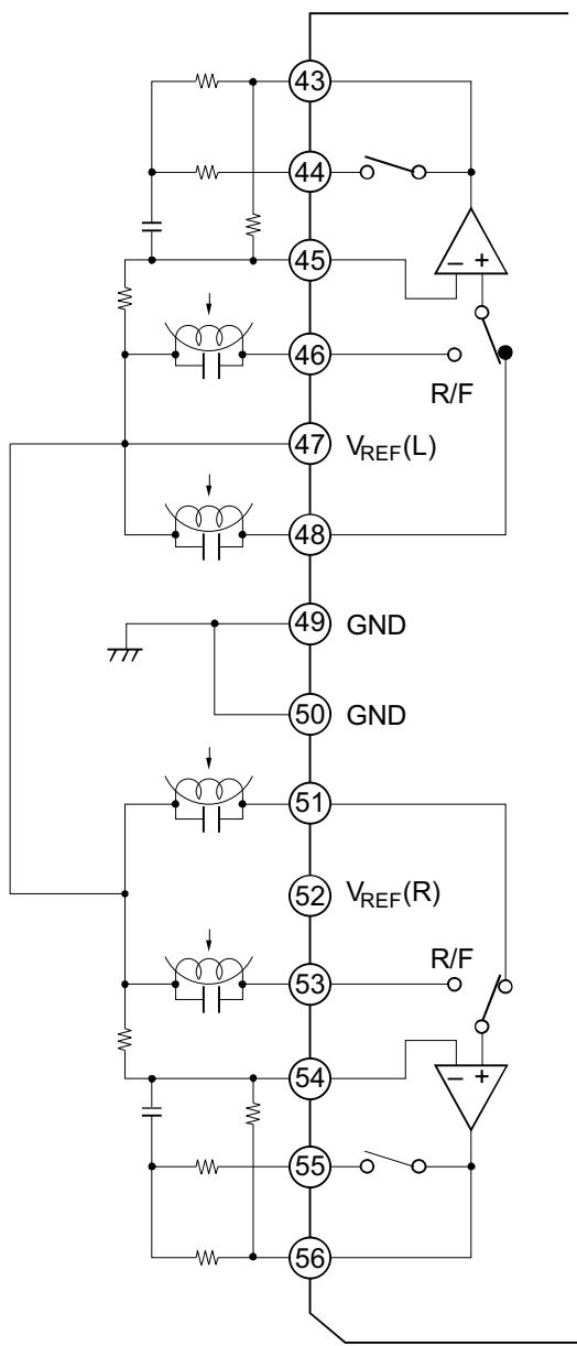
**Figure 3 Application Circuit**
