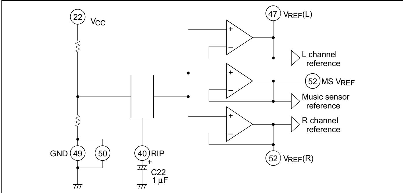
**Figure 1** The Block Diagram of Reference Voltage Supply
