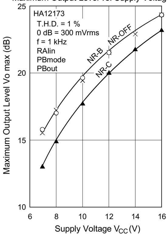
Maximum Output Level vs. Supply Voltage (2)
