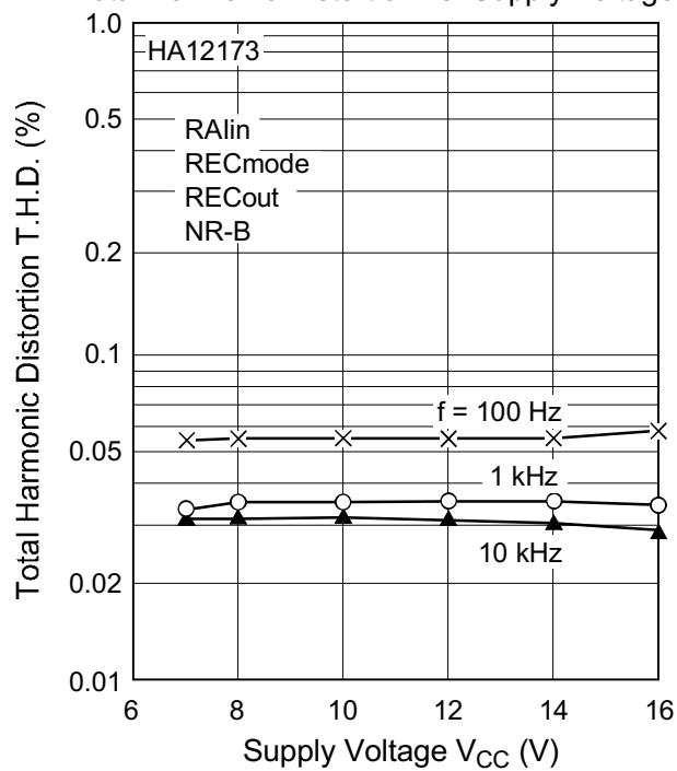
Total Harmonic Distortion vs. Supply Voltage (6)
