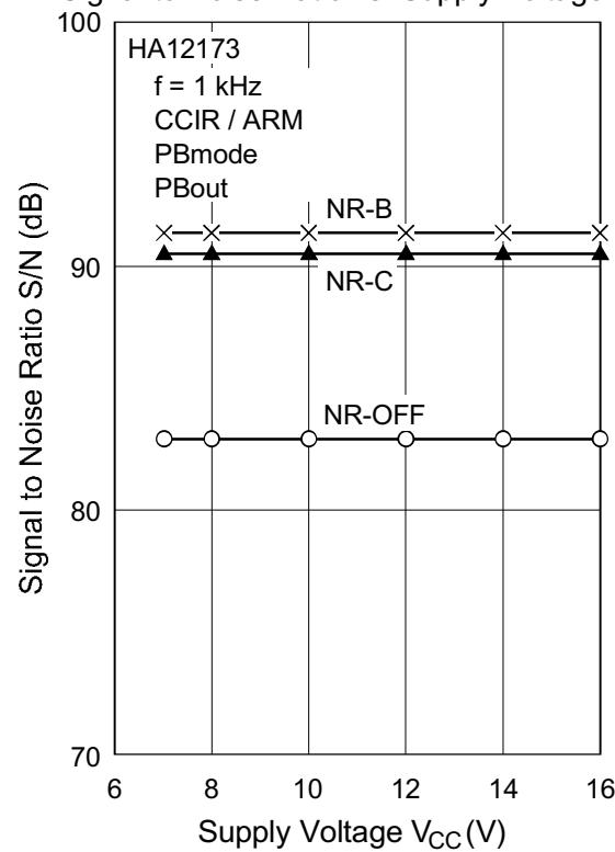
Signal to Noise Ratio vs. Supply Voltage (2)
