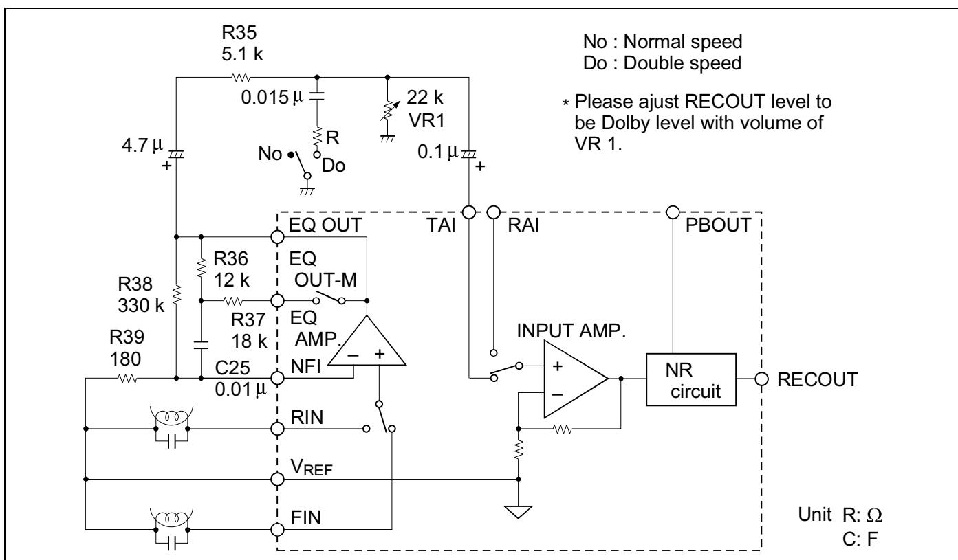
Figure 7 Application Circuit for Double Speed
