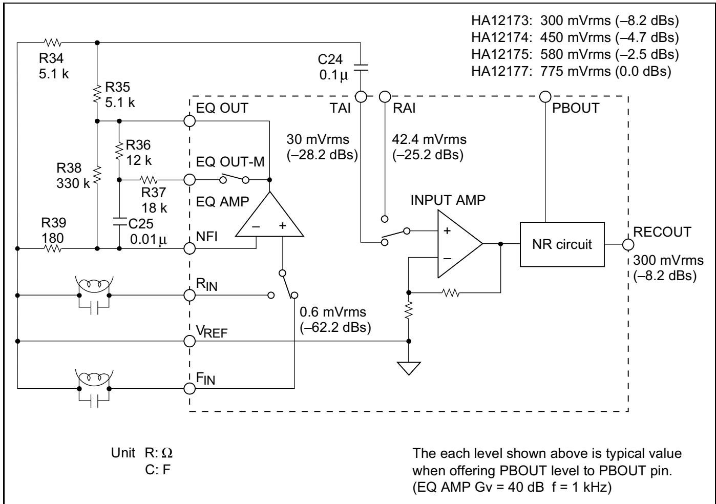
**Figure 2 Input Block Diagram**
