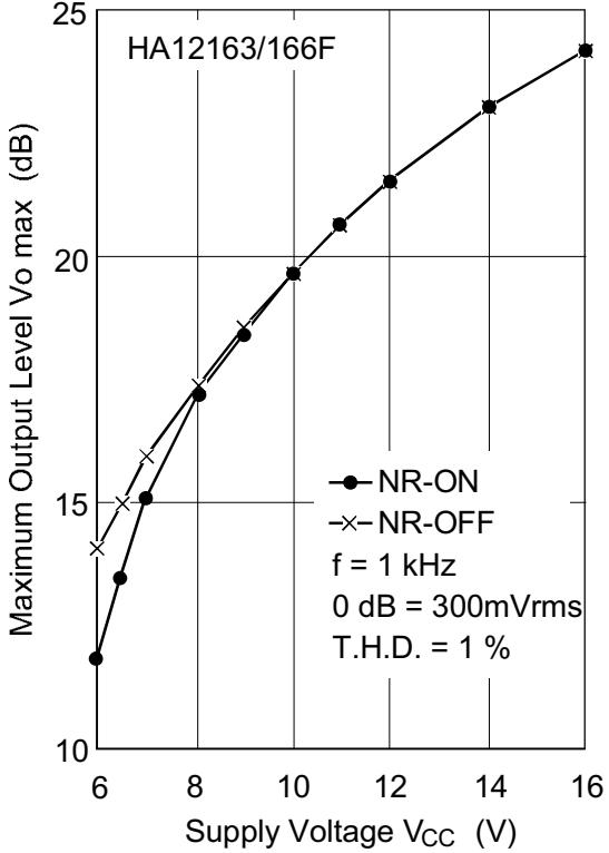
Maximum Output Level vs. Supply Voltage (2)
