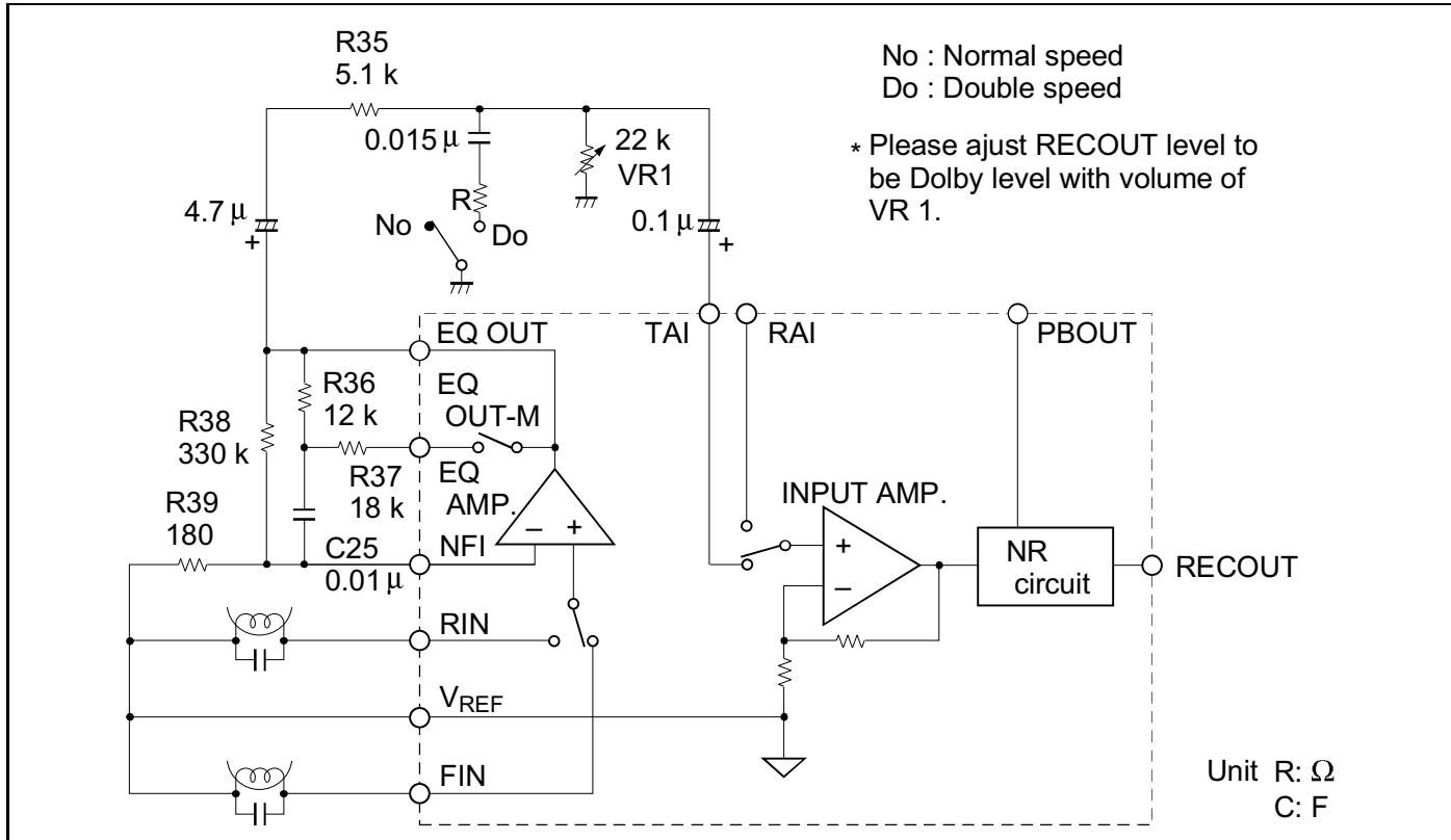
Figure 7 Application Circuit for Double Speed
