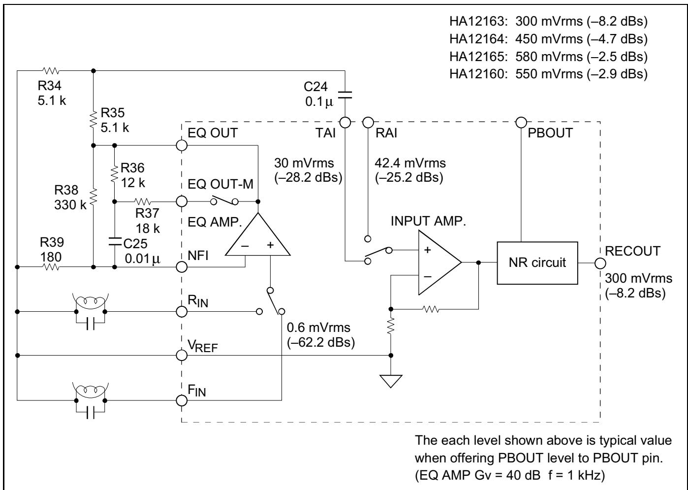
**Figure 2 Input Block Diagram**
