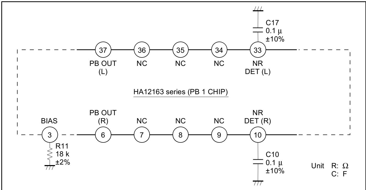
**Figure 6 Tolerances of External Components**
