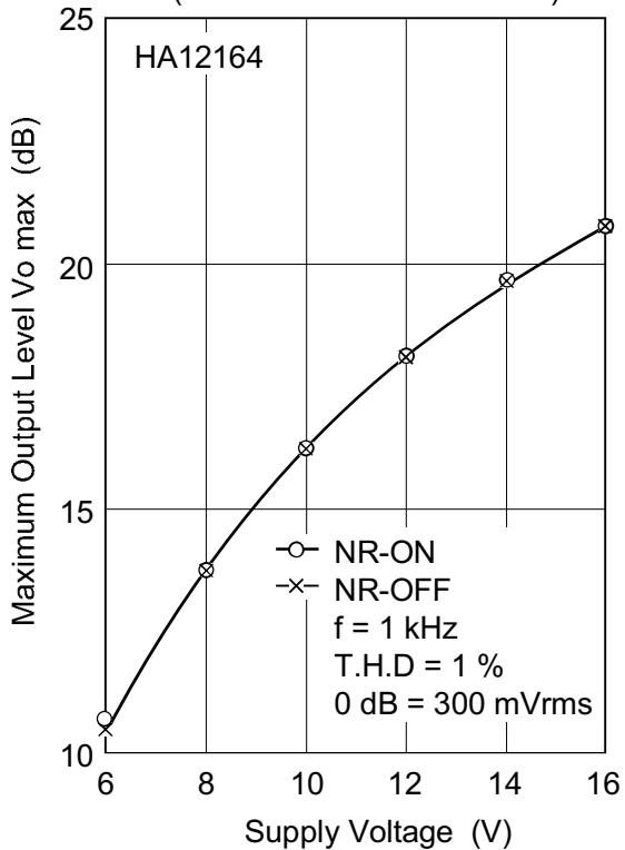
Maximum Output Level vs. Supply Voltage (2)
