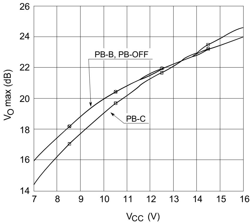
**Maximum Output Level vs. Supply Voltage (PB MODE)****HA12141NT, HA12161FP**
