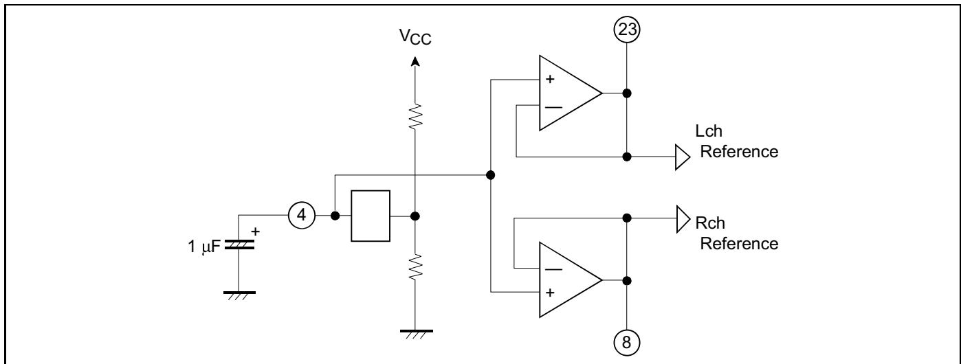
**Figure 1 The Block-Diagram of Reference Voltage Supply**
