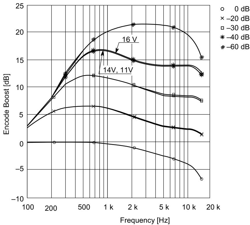
**Encode Boost vs. Frequency (NR-C  $V_{cc}$  = 11 V, 14 V, 16 V)**
