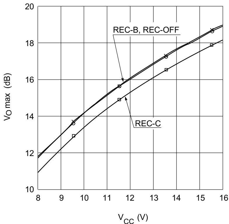
**Maximum Output Level vs. Supply Voltage (REC MODE)****HA12142NT, HA12162FP**
