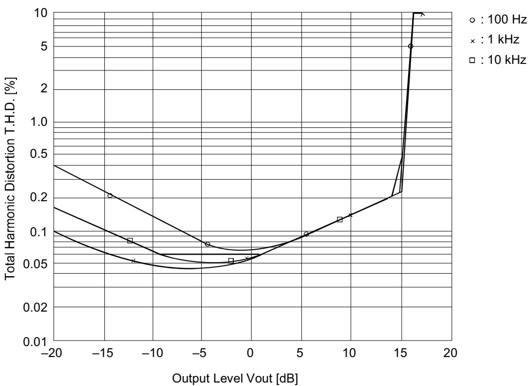
**Total Harmonic Distortion vs. Output Level (PB MODE NR-B V<sub>cc</sub> = 14 V)**
