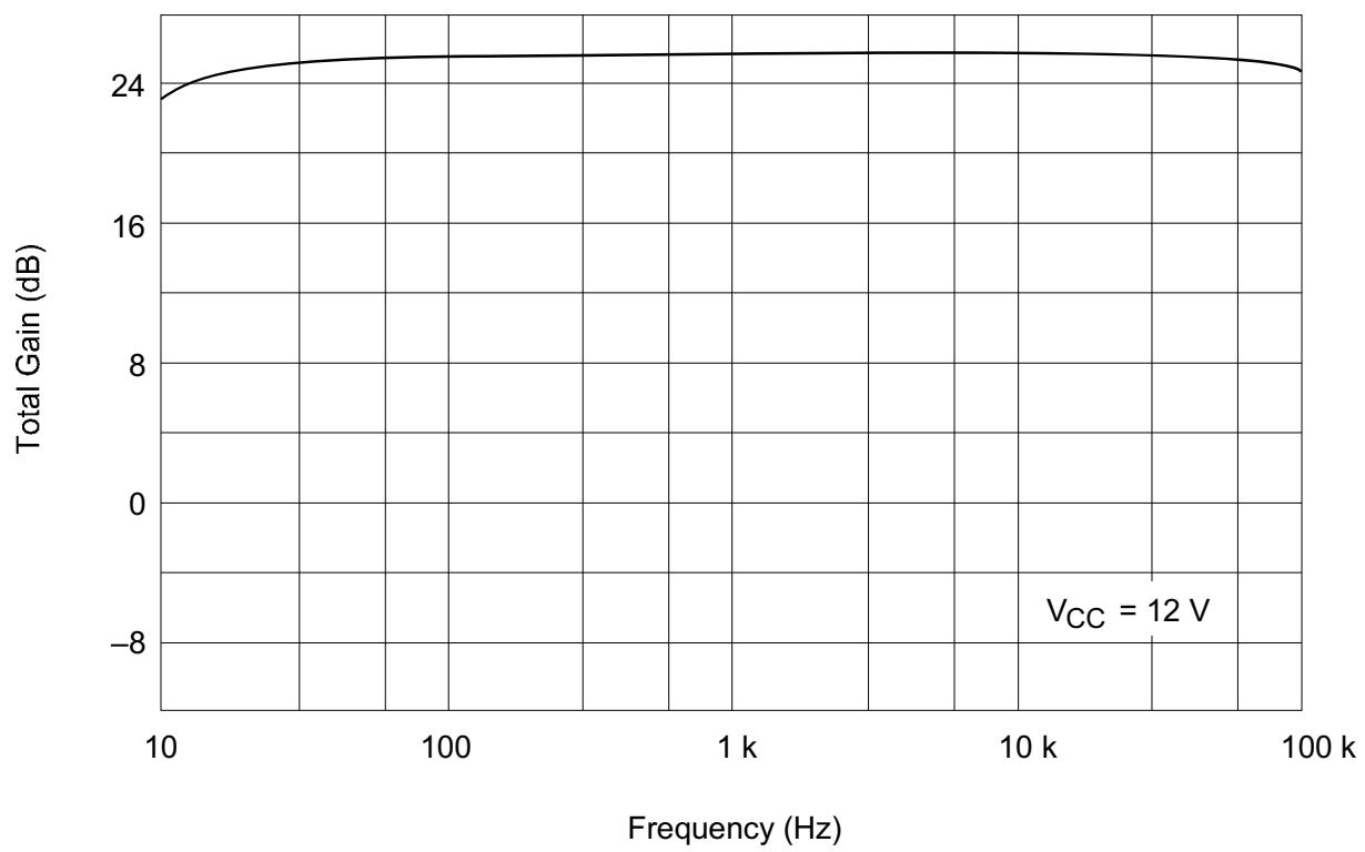
**Total Gain vs. Frequency (PB MODE POUT NR-OFF)**
