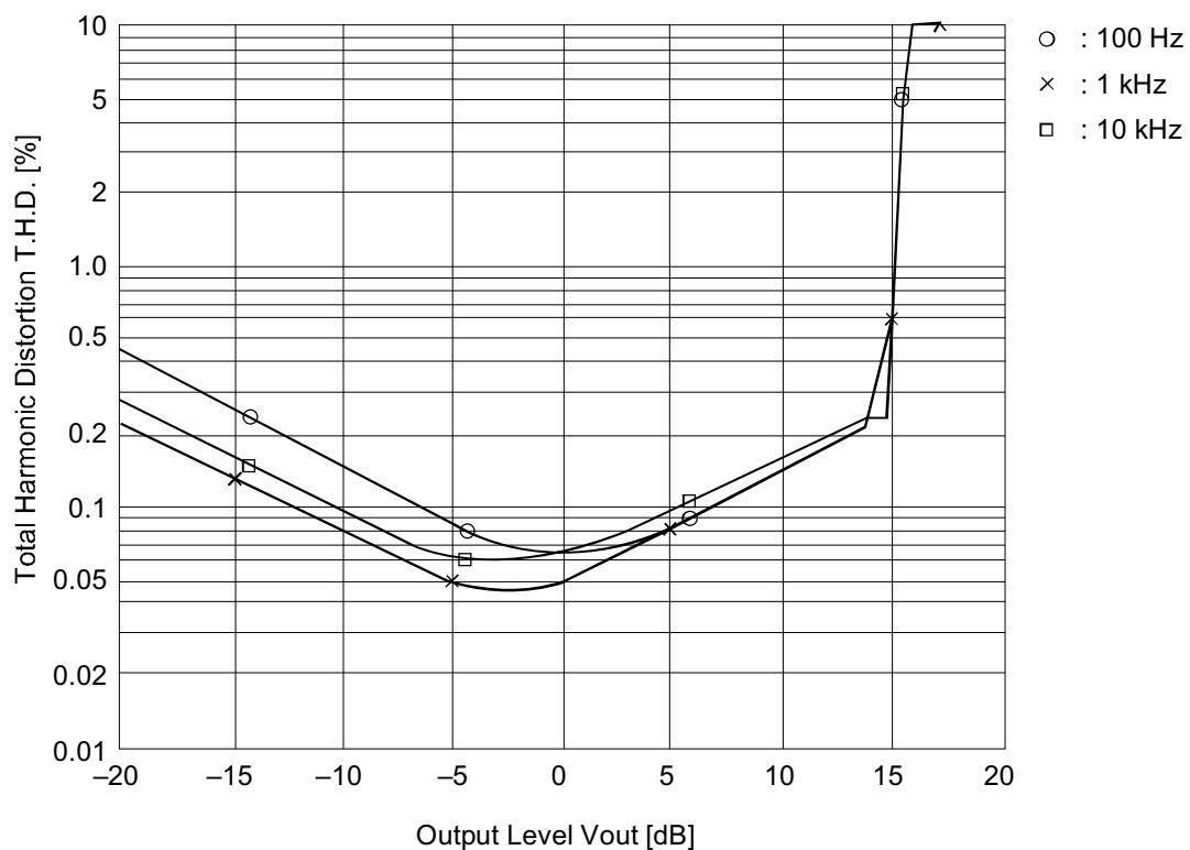
**Total Harmonic Distortion vs. Output Level (PB MODE NR-OFF V<sub>cc</sub> = 14 V)**
