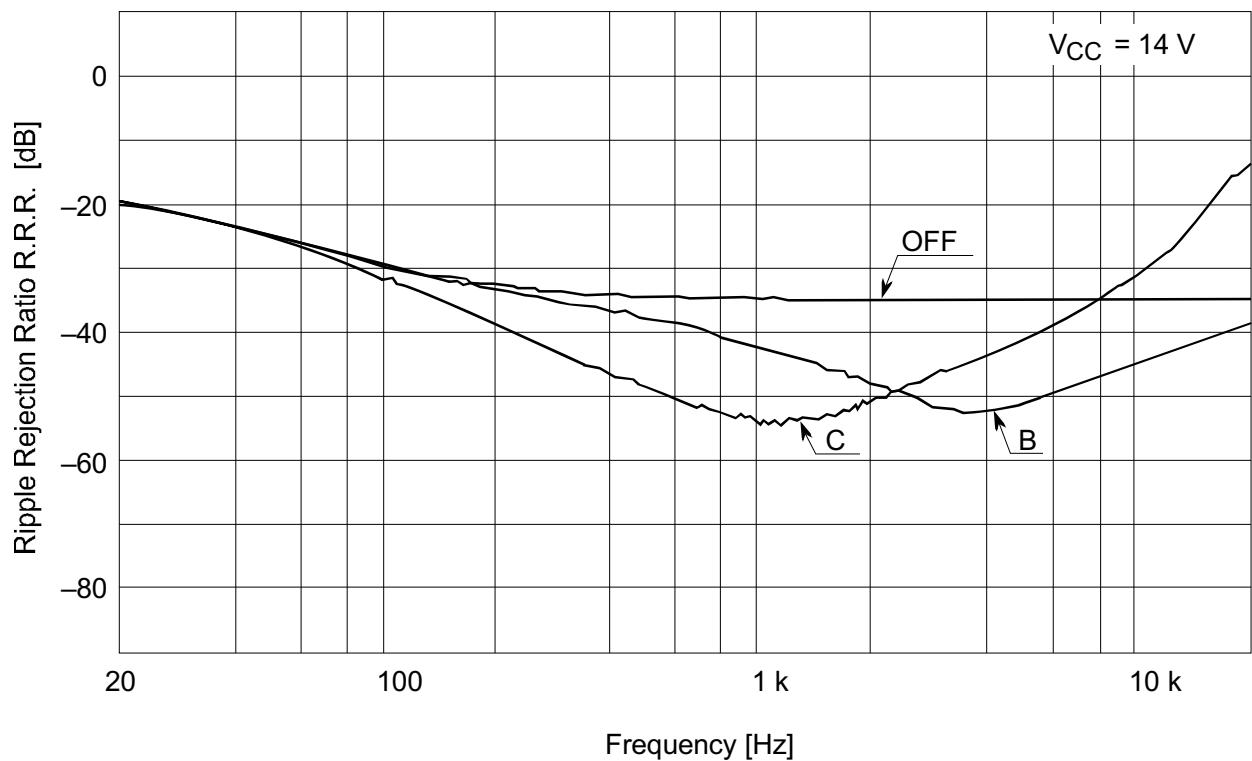
**Ripple Rejection Ratio vs. Frequency (PB MODE PBOOT)**
