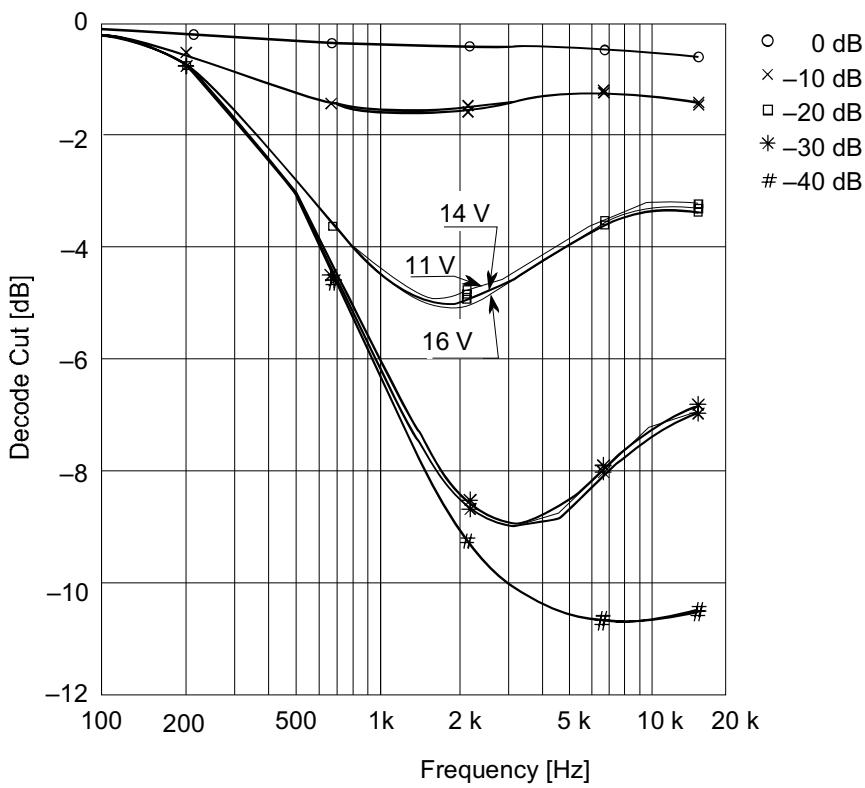
**Decode Cut vs. Frequency (NR-B  $V_{cc}$  = 11 V, 14 V, 16 V)**
