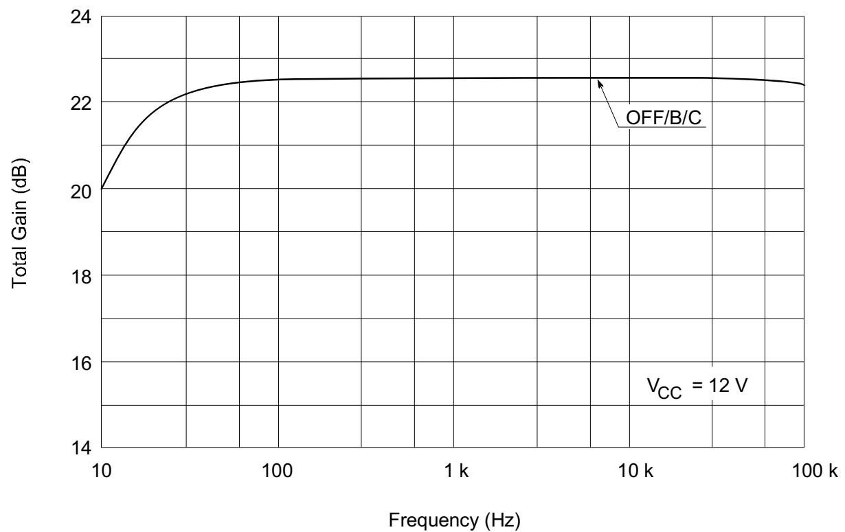
**Total Gain vs. Frequency (REC MODE PBOUT)**
