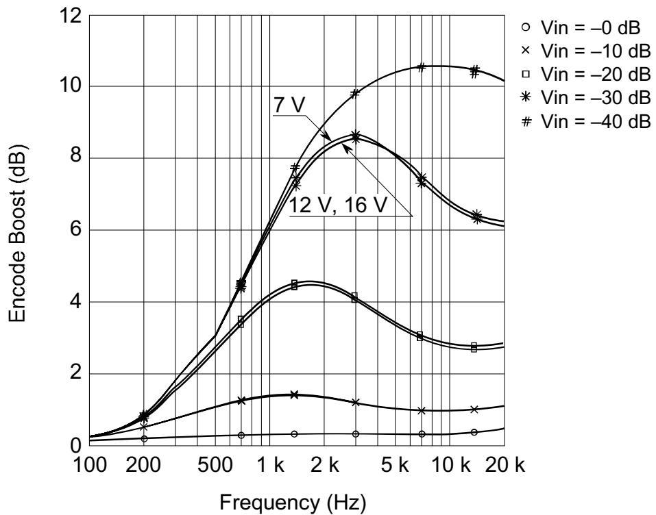
Encode Boost vs. Frequency (NR-B V<sub>cc</sub> = 7V, 12 V, 16 V)
