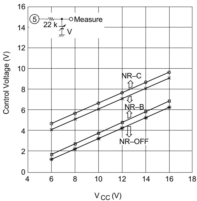
Control Voltage vs. Supply voltage (NR-OFF/B/C)
