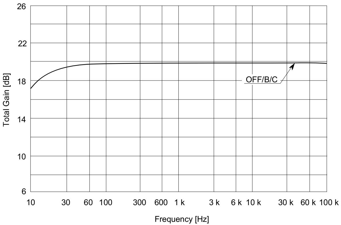
**Total Gain vs. Frequency (PB MODE RECOUT  $V_{cc} = 14$  V)**
