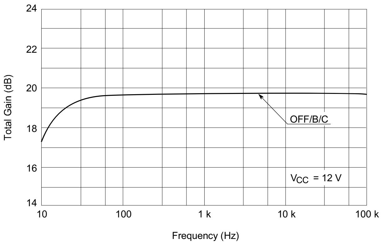
**Total Gain vs. Frequency (PB MODE RECOUT)**
