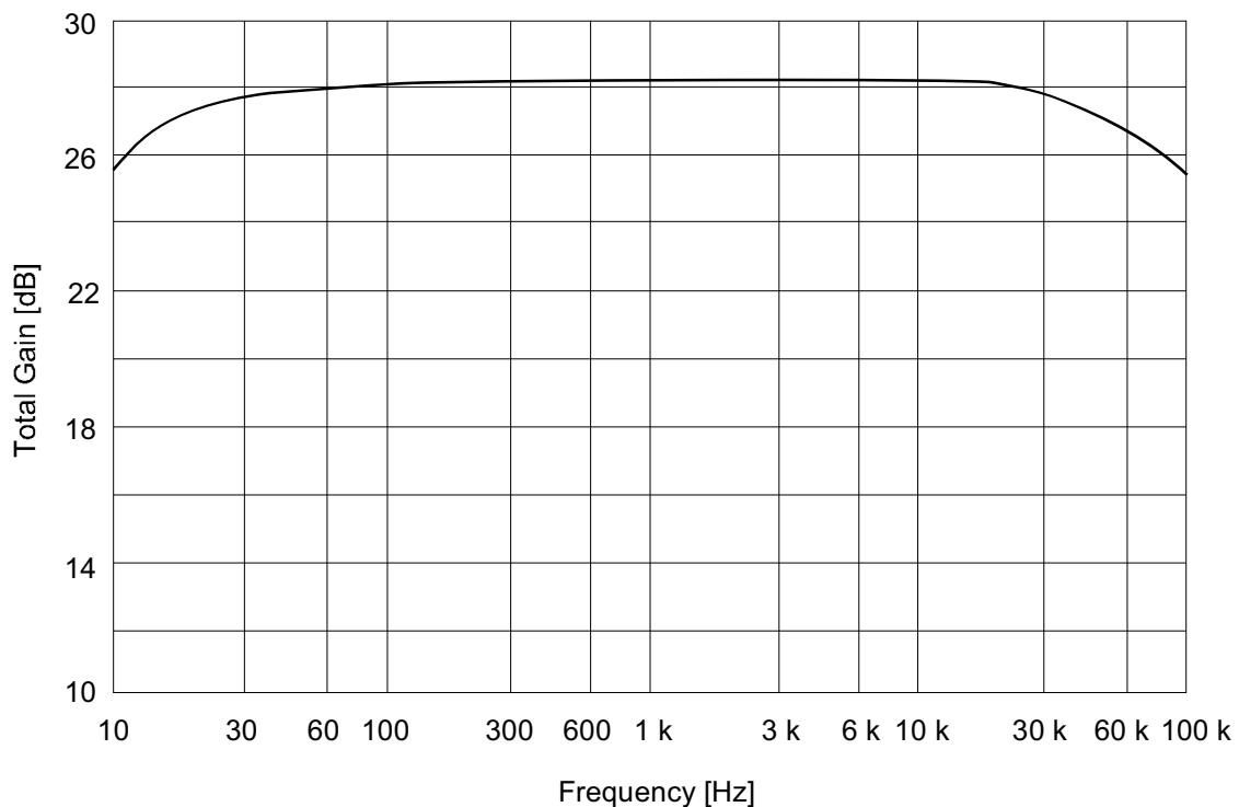
**Total Gain vs. Frequency (PB MODE POUT NR-OFF  $V_{cc} = 14$  V)**
