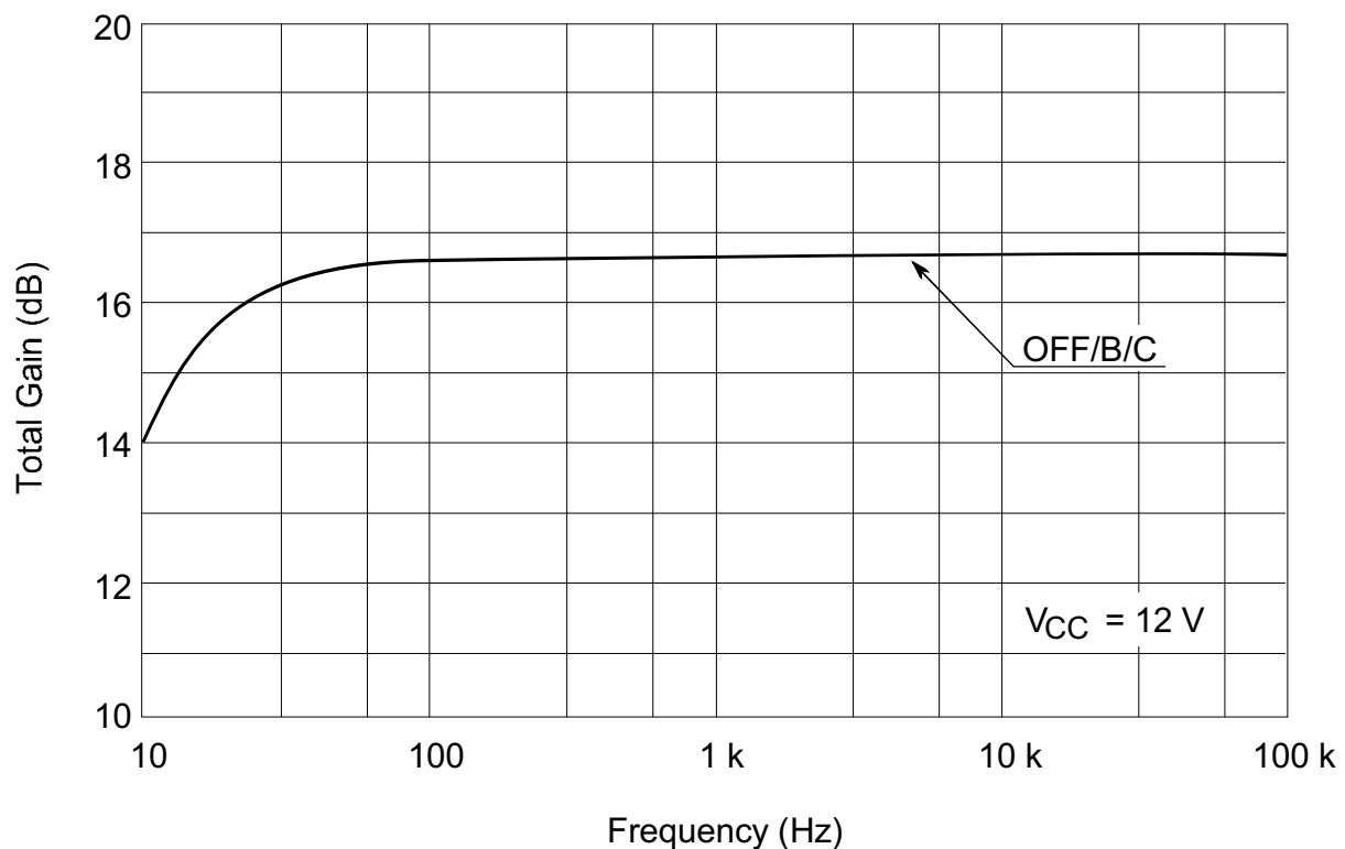
**Total Gain vs. Frequency (REC MODE PBOUT)**
