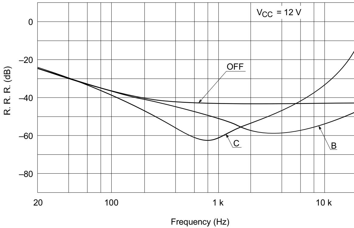
**Ripple Rejection Ratio vs. Frequency (PB MODE POUT)**
