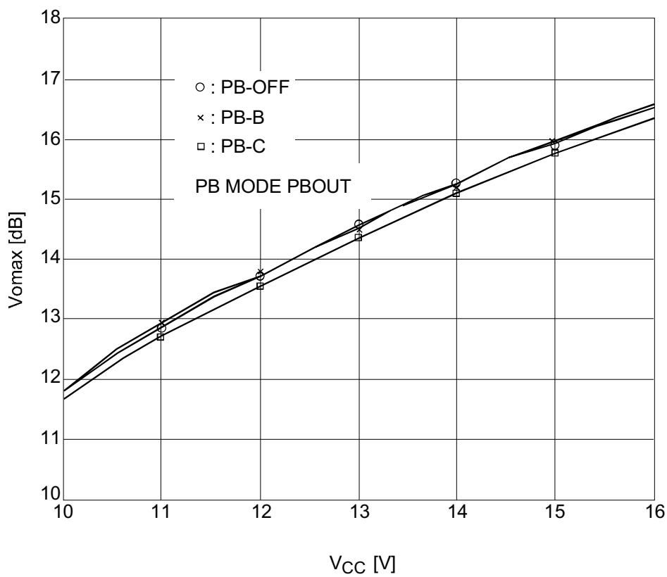
**Maximum Output Level vs. Supply Voltage**
