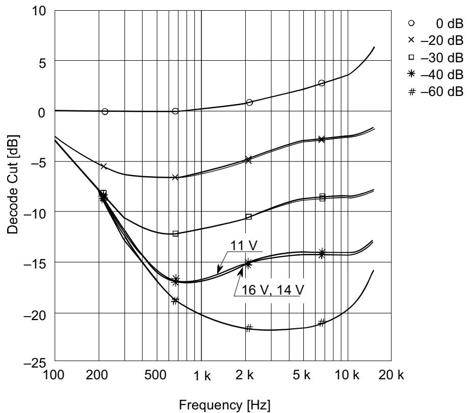
**Decode Cut vs. Frequency (NR-C  $V_{cc} = 11\text{ V}, 14\text{ V}, 16\text{ V}$ )**
