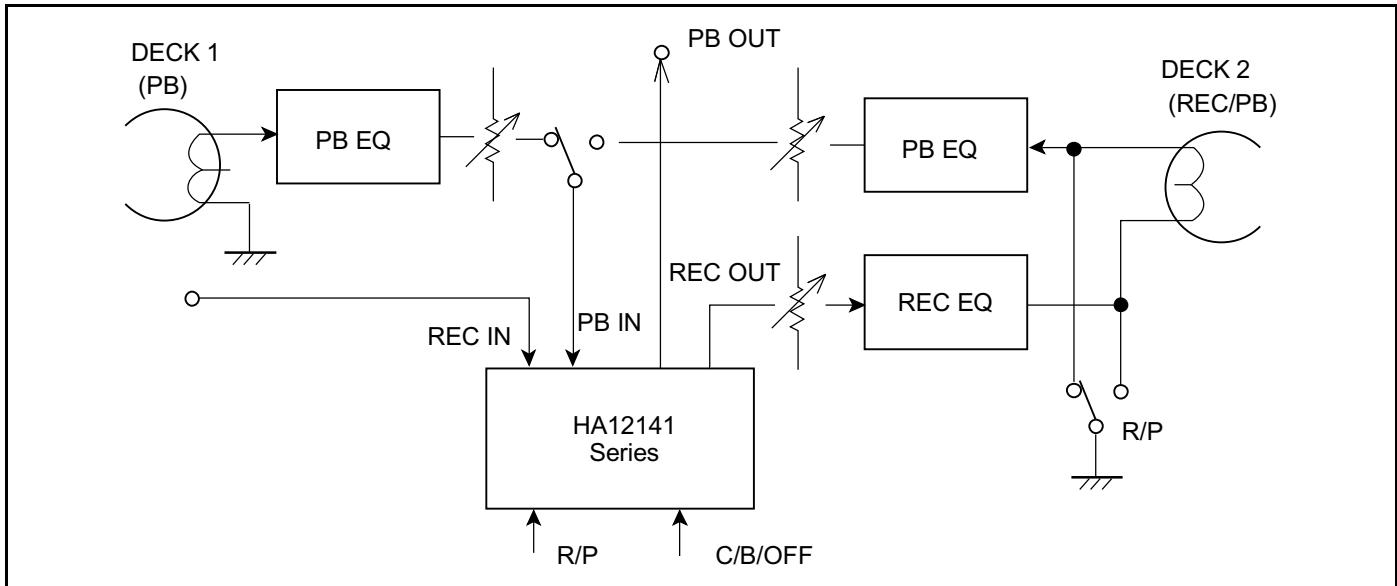
**Figure 5 Application for Dubbing Deck**
