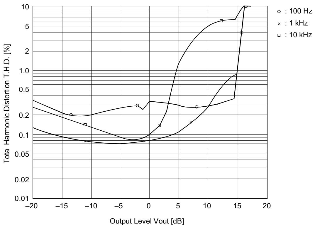
**Total Harmonic Distortion vs. Output Level (PB MODE NR-C V<sub>cc</sub> = 14 V)**
