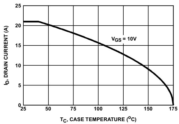
FIGURE 2. MAXIMUM CONTINUOUS DRAIN CURRENT vs
