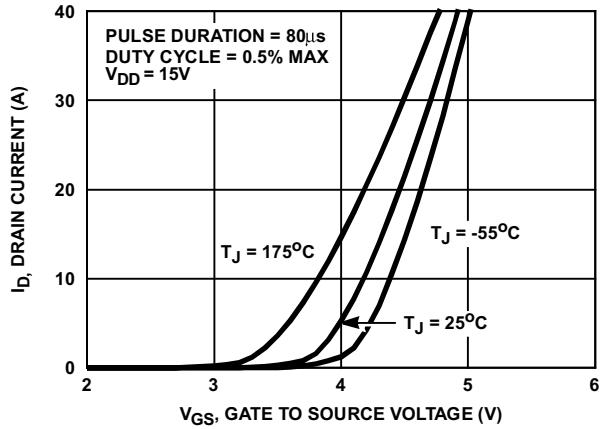
FIGURE 7. TRANSFER CHARACTERISTICS
