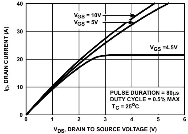
FIGURE 8. SATURATION CHARACTERISTICS
