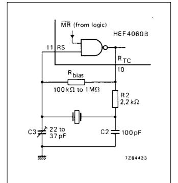
Fig.5 External component connection for crystal oscillator.
