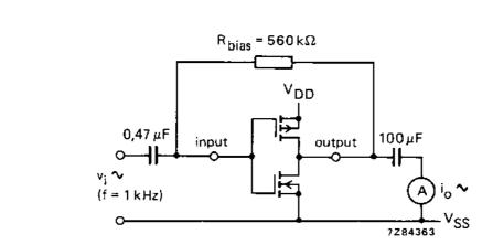
Fig.6 Test set-up for measuring forward transconductance  $g_{fs} = di_o/dv_i$  at  $v_o$  is constant (see also graph Fig.7); MR = LOW.
