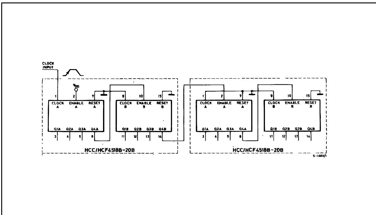
**TYPICAL APPLICATION****SYNCHRONOUS CASCADING OF 4 BINARY COUNTERS WITH NEGATIVE-EDGE TRIGGERING**
