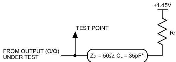
\*C<sub>L</sub> includes test fixture and probe capacitance.
