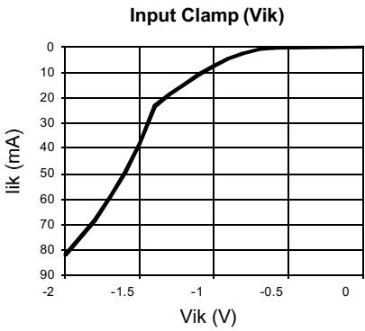
**GAL16V8D-7 (Except IND PLCC)/-10L: Typical AC and DC Characteristic Diagrams**
