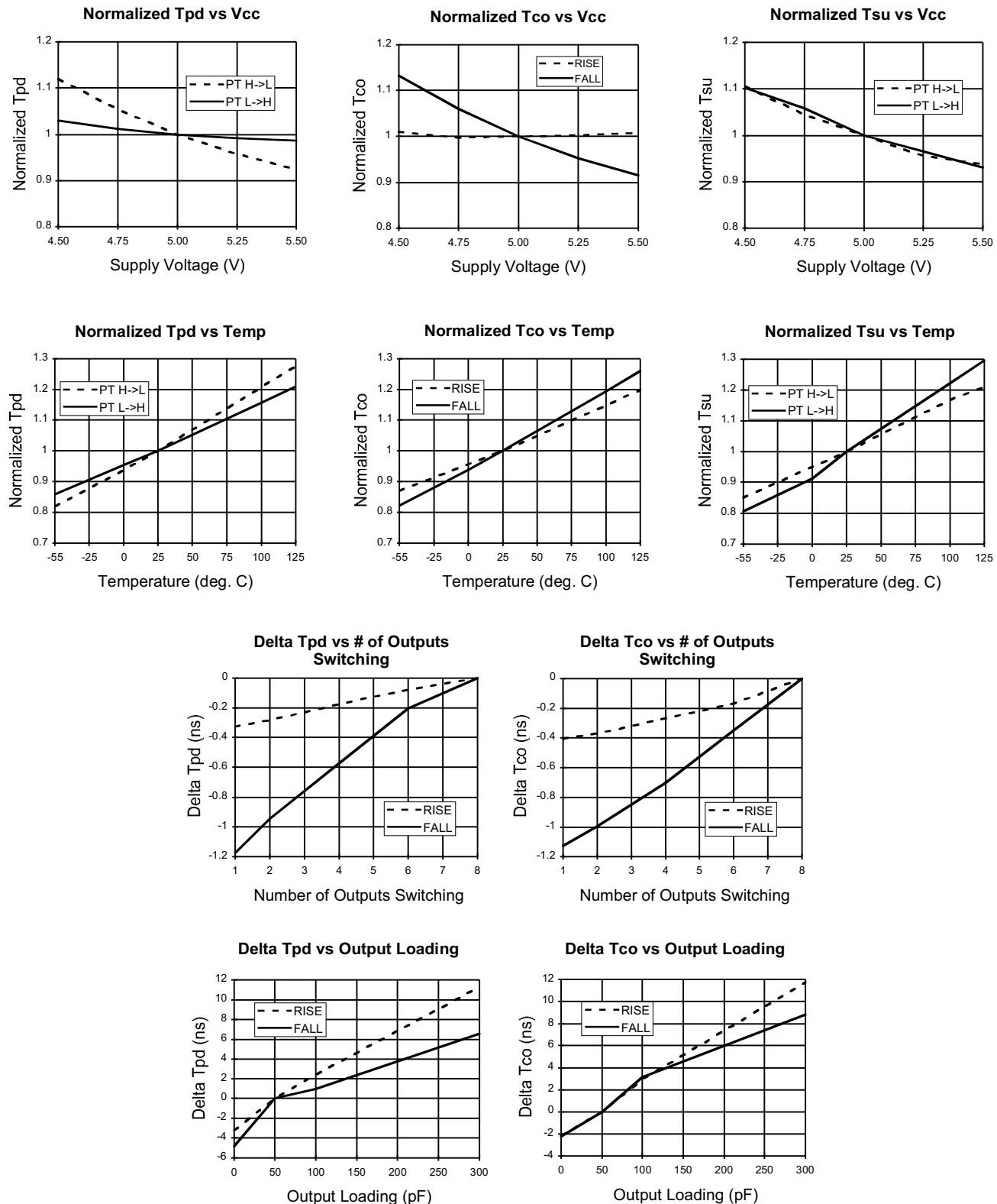
**GAL16V8D-10Q (and Slower): Typical AC and DC Characteristic Diagrams**
