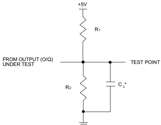
\*C<sub>L</sub> INCLUDES TEST FIXTURE AND PROBE CAPACITANCE
