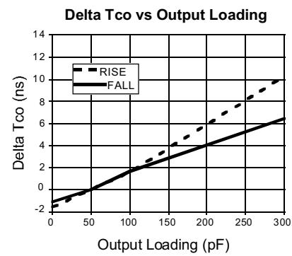
**GAL16V8D-3/-5/-7 (IND PLCC): Typical AC and DC Characteristic Diagrams**
