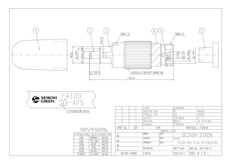
S07-038-4E FC/SC Plug Type Fixed Attenuator
