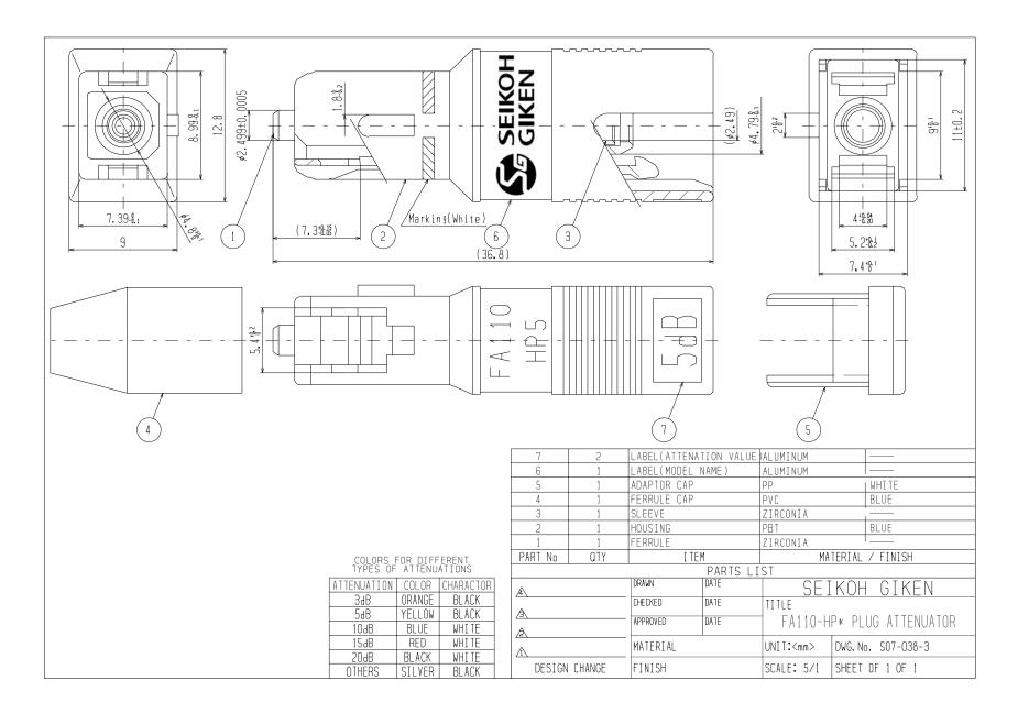
S07-038-4E FC/SC Plug Type Fixed Attenuator
