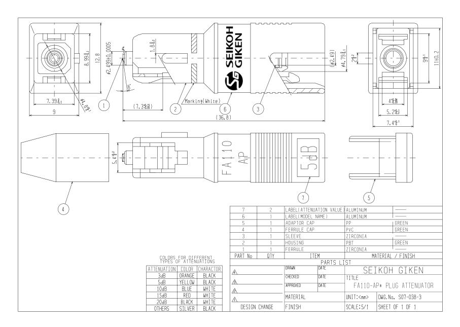
S07-038-4E FC/SC Plug Type Fixed Attenuator
