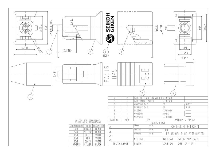
S07-038-4E FC/SC Plug Type Fixed Attenuator
