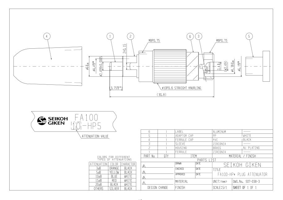
S07-038-4E FC/SC Plug Type Fixed Attenuator
