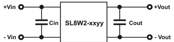
It is necessary to add the Cin and Cout of low ESR capacitors for application and testing.
