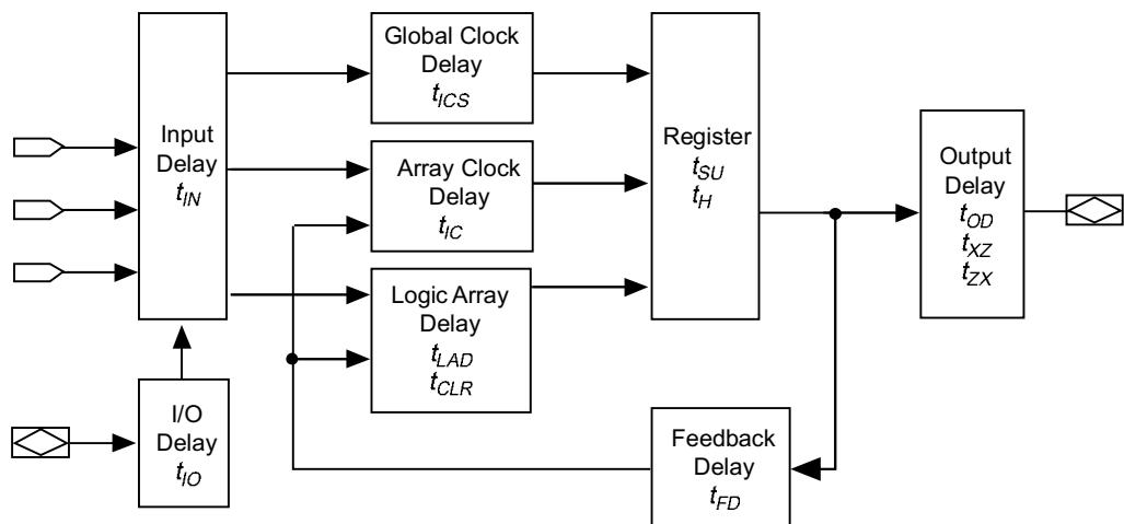
Timing information can be derived from the timing model and parameters for a particular device. External timing parameters represent pin-to-pin timing delays, and can be calculated from the sum of internal parameters. [Figure 5](#) shows the internal timing relationship for internal and external delay parameters.
