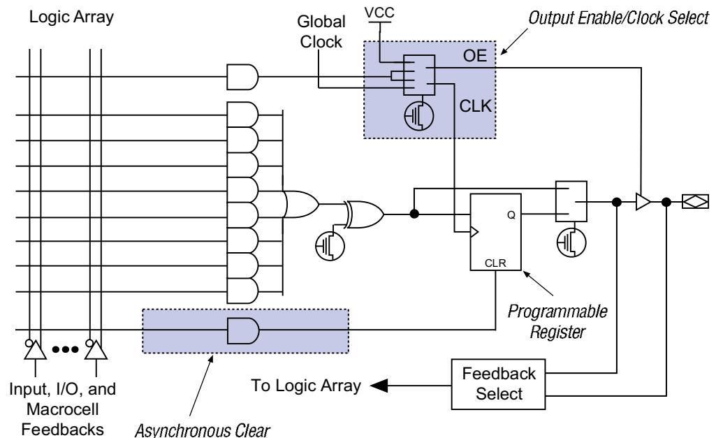
The eight product terms of the programmable-AND array feed the 8-input OR gate, which then feeds one input to an XOR gate. The other input to the XOR gate is connected to a programmable bit that allows the array output to be inverted. Altera's MAX+PLUS II software uses the XOR gate to implement either active-high or active-low logic, or De Morgan's inversion to reduce the number of product terms needed to implement a function.
