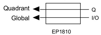
EP610, EP610I, EP910, and EP910I devices have a global feedback configuration; either the macrocell output (Q) or the I/O pin input (I/O) can feed back to the AND array so that it is accessible to all other macrocells.
