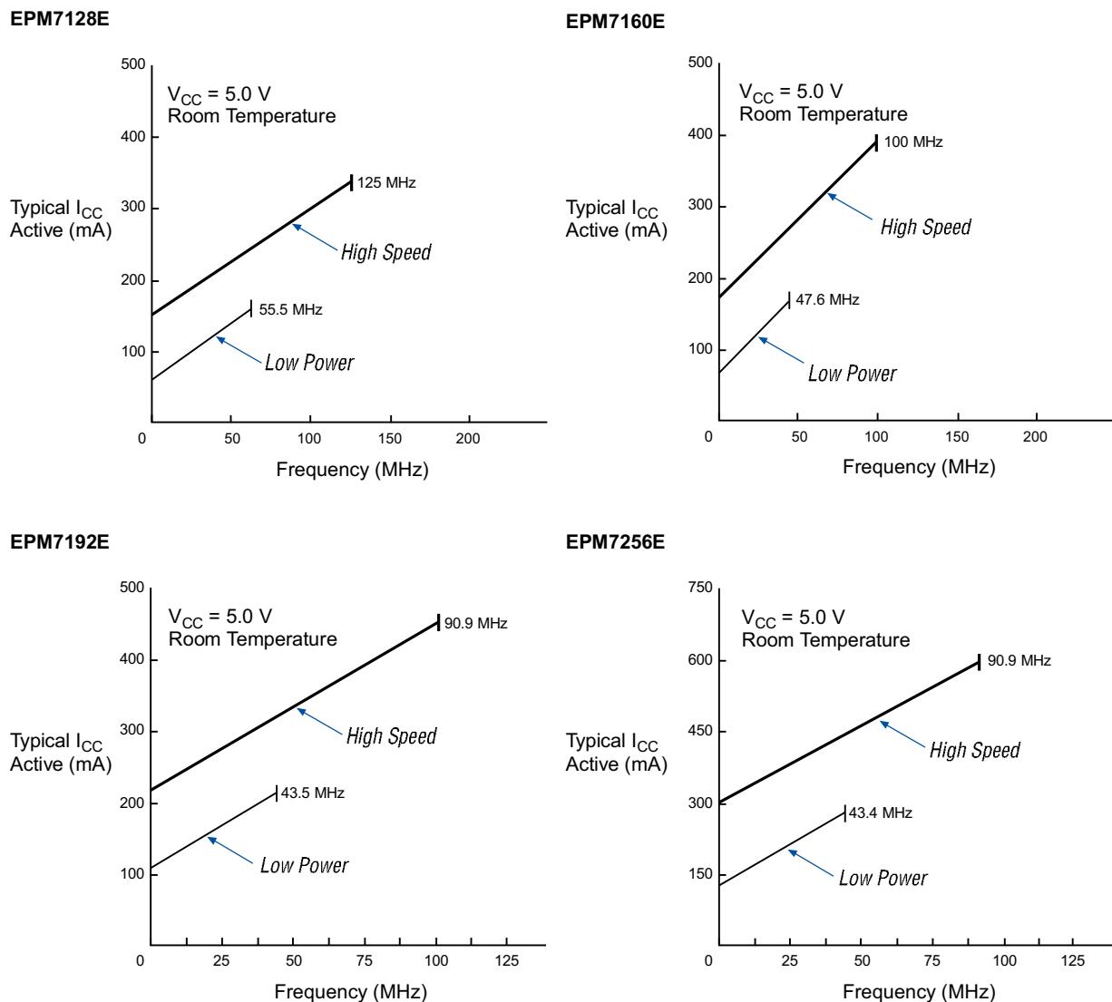
**Figure 15** shows typical supply current versus frequency for MAX 7000S devices.
