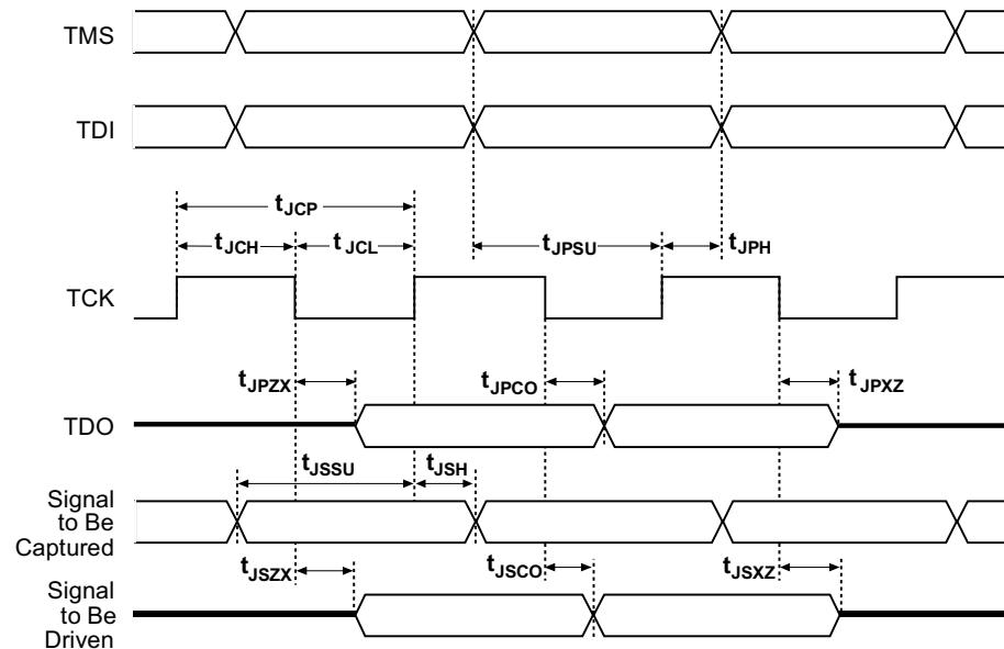
Table 12 shows the JTAG timing parameters and values for MAX 7000S devices.
