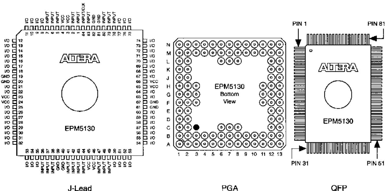
The EPM5130 EPLD is available in windowed ceramic 84-pin J-lead chip carrier (JLCC), 100-pin pin-grid array (PGA), and 100-pin quad flat pack (QFP) packages, as well as OTP plastic J-lead (PLCC) and QFP packages.
