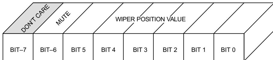
**DS1807 ATTENUATOR CONFIGURATION** Figure 3
