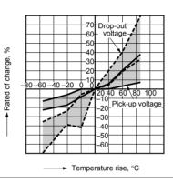
4.-(2) Pick-up/drop-out voltage vs. temperature (1-coil latching) Sample: DR-L-5V, 5 pcs.
