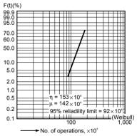
6.-(2) Electrical life test Sample 10 pcs. DR-12V Load: 101 mA 53 V DC relay coil 2 pcs. HG4-DC48V coils in parallel
