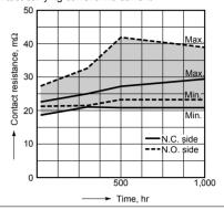
3.-(2) Leaving at high temperature (Change of pick-up and drop-out voltages) Tested Sample: DR-24V, 10pcs Ambient temperature: 85°C 185°F Coil applied voltage: 24V DC (Nominal voltage) Contact carrying current: No current
