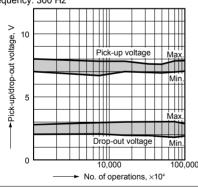
5.-(2) Mechanical life Change of contact resistance Sample: DR-12V, 5 pcs. Frequency: 300 Hz
