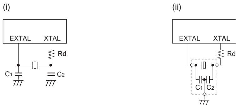
Fig. 13. Recommended Oscillation circuit
