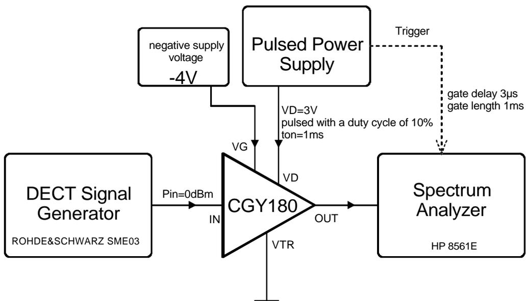
\*)measured with a CGY180 test circuit board (see page 11) VD=3V, VG=-4V, VTR=0V
