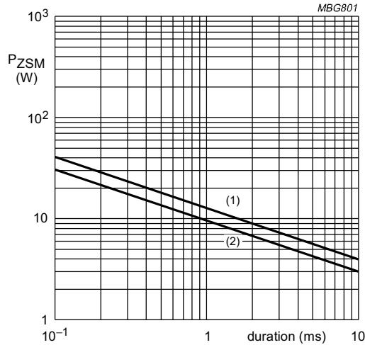
Fig.3 Maximum permissible non-repetitive peak reverse power dissipation versus duration.
