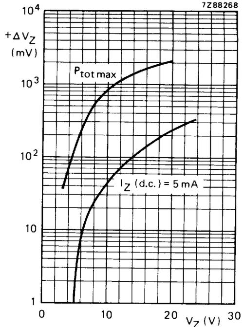
Fig. 12 Typical change of working voltage;
