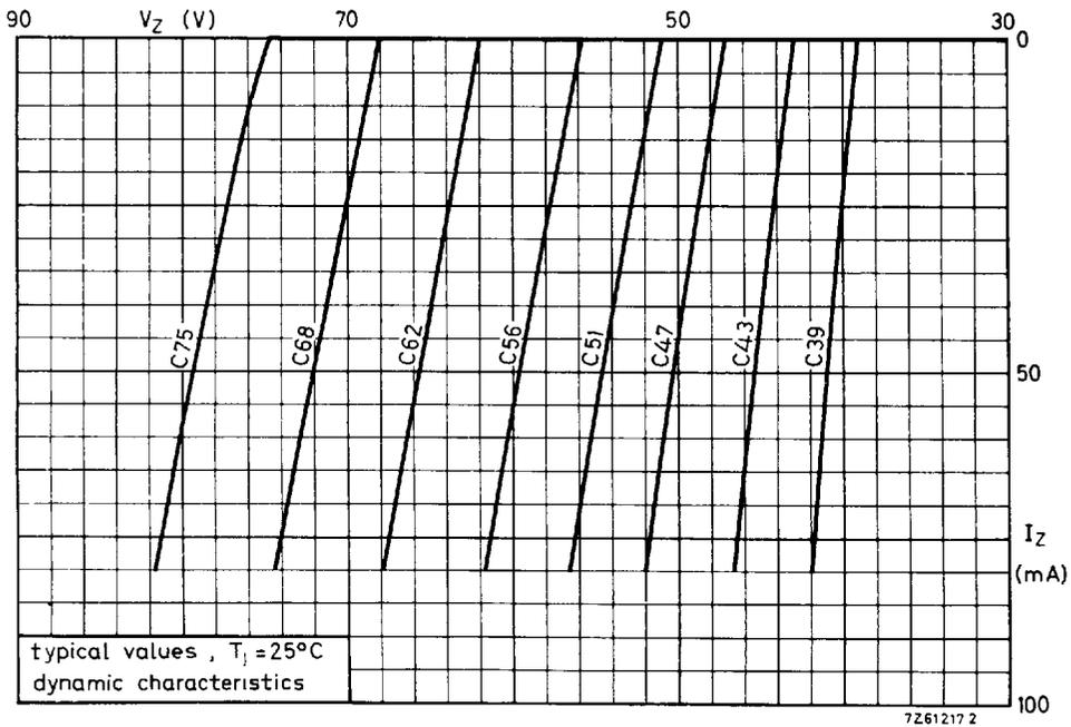
Fig. 5 Dynamic characteristics; typical values at  $T_j = 25^\circ\text{C}$ .
