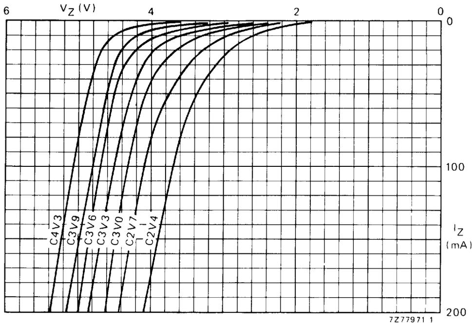
Fig. 2 Dynamic characteristics; typical values;  $T_j = 25^\circ\text{C}$ .
