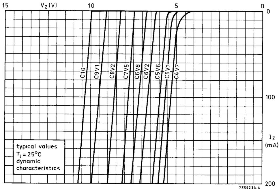
Fig. 3 Dynamic characteristics; typical values at  $T_j = 25^\circ\text{C}$ .
