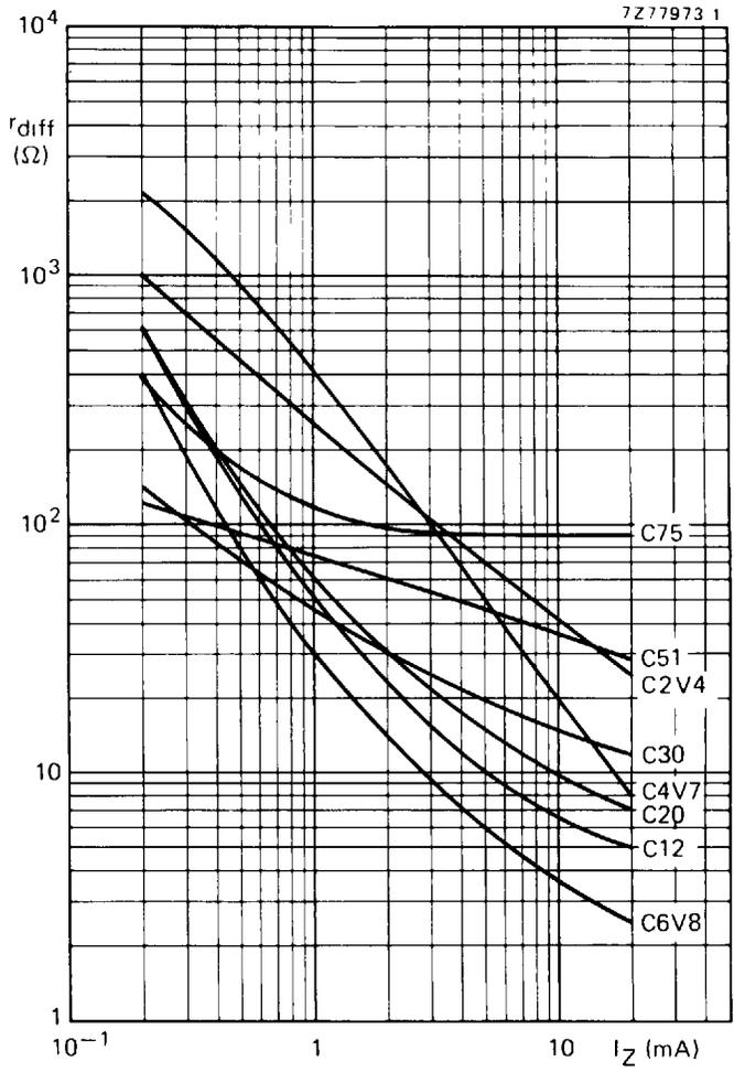
Fig. 14 Typical values;  $T_j = 25^\circ\text{C}$ ;  $f = 1\text{ kHz}$ .
