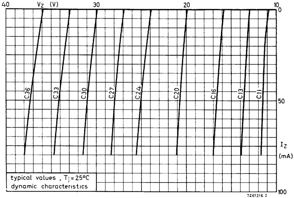
Fig. 4 Dynamic characteristics; typical values;  $T_j = 25^\circ\text{C}$ .
