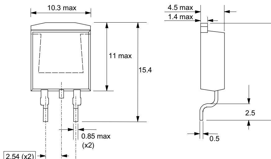
Fig.18. SOT404 : centre pin connected to mounting base.
