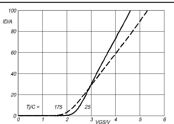
Fig.7. Typical transfer characteristics.
