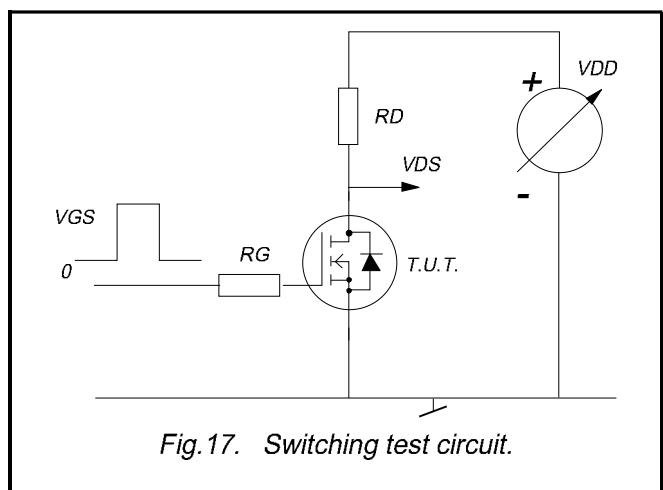
*Fig.17. Switching test circuit.*
