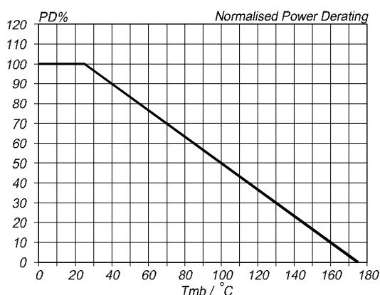
Fig. 1. Normalised power dissipation.
