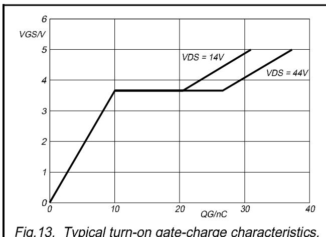
Fig.13. Typical turn-on gate-charge characteristics.
