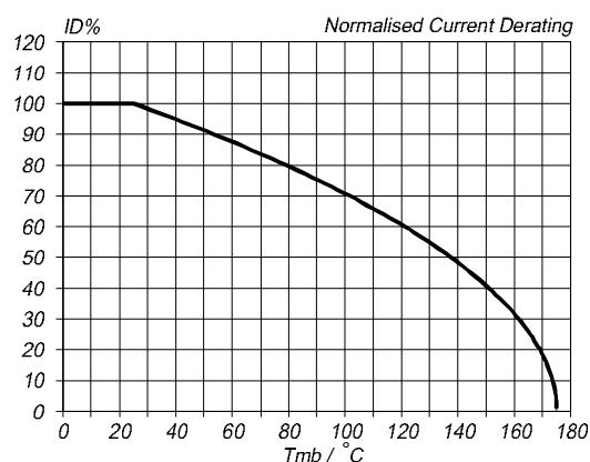
Fig. 2. Normalised continuous drain current.
