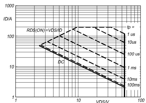
Fig. 3. Safe operating area.  $T_{mb} = 25^\circ\text{C}$
