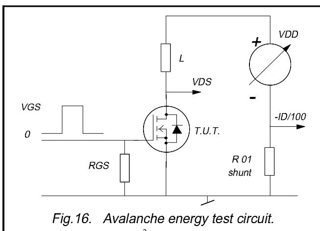
Fig.16. Avalanche energy test circuit.
