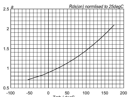
Fig.9. Normalised drain-source on-state resistance.
