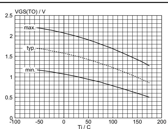
Fig.10. Gate threshold voltage.
