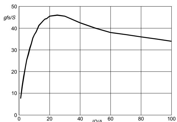
Fig.8. Typical transconductance,  $T_j = 25^\circ\text{C}$ .
