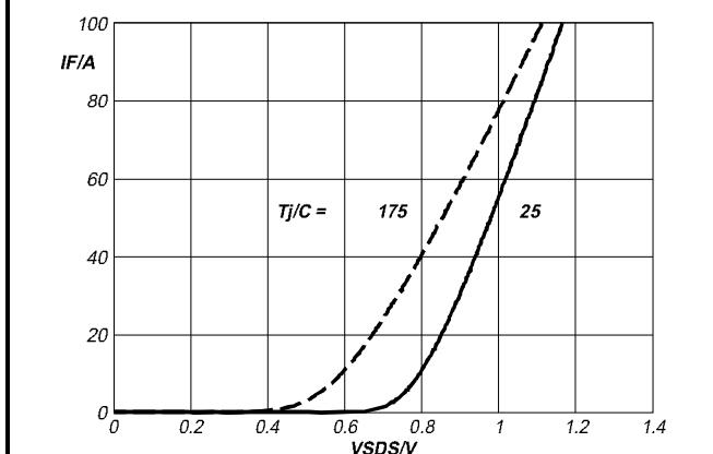
Fig.14. Typical reverse diode current.
