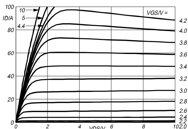
Fig.5. Typical output characteristics,  $T_j = 25^\circ\text{C}$ .
