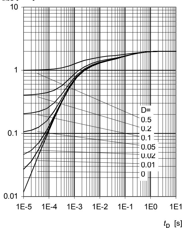
**Transient thermal impedance chip case**
