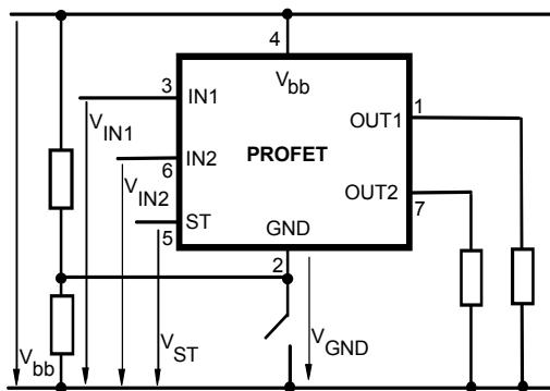
Any kind of load. If  $V_{GND} > V_{IN} - V_{IN(T+)}$  device stays off. Due to  $V_{GND} > 0$ , no  $V_{ST} = \text{low}$  signal available.
