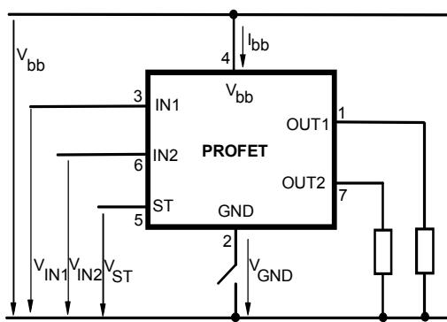
Any kind of load. In case of Input=high is  $V_{OUT} \approx V_{IN} - V_{IN(T+)}$ . Due to  $V_{GND} > 0$ , no  $V_{ST} = \text{low}$  signal available.
