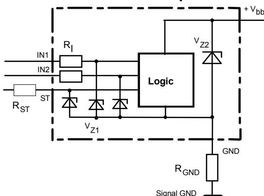
$V_{Z1} = 6.1$  V typ.,  $V_{Z2} = 47$  V typ.,  $R_I = 3.5 \text{ k}\Omega$  typ,
