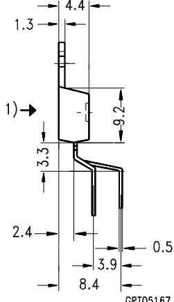
1) shear and punch direction no burrs this surface
