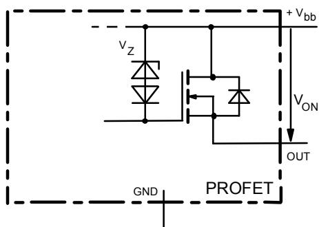
$V_{ON}$  clamped to 47 V typ.
