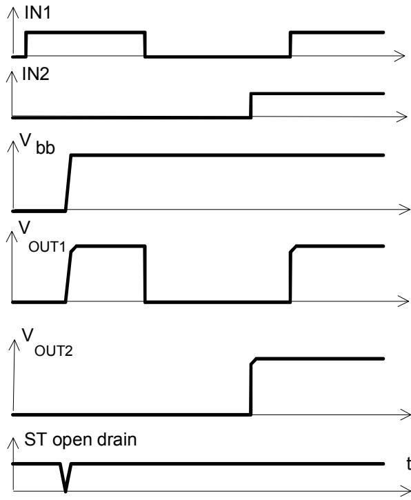
**Figure 2b:** Switching an inductive load
