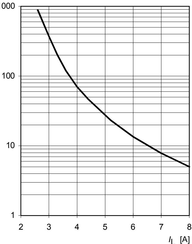
**Typ. transient thermal impedance chip case**
