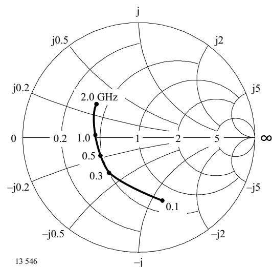
Figure 4. Input reflection coefficient
